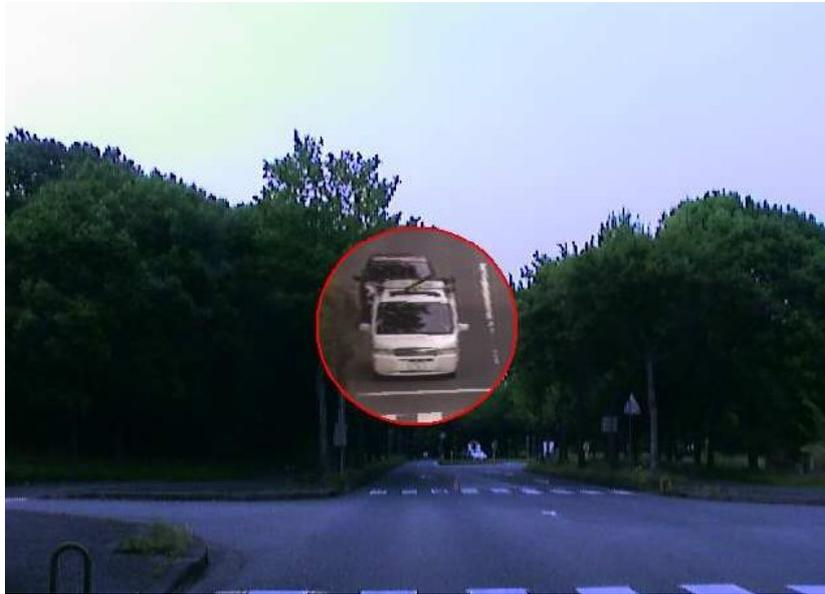
Figure 4.8: Virtual Back Mirror floating in the HUD showing the correctly transformed view of a fixed camera on the street; courtesy of [113]
