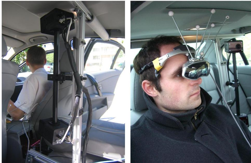
(a) Snapshot of the two tracking cameras from behind and the covered tracking volume (b) The HMD worn in the tracking volume. The tracking cameras (back right) can see the markers
