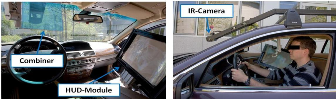
(a) Photography of the internal setup of the HUD system; courtesy of [20] (b) Photography of the mounting of the infrared camera; courtesy of [20]
