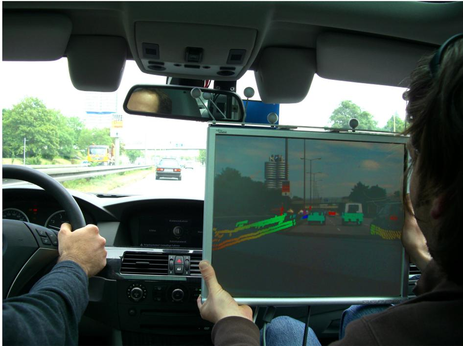
Figure 9.11: The TFT held into the tracking volume while driving. One can see the laser-scanner augmentation on the vehicles and the guardrail
