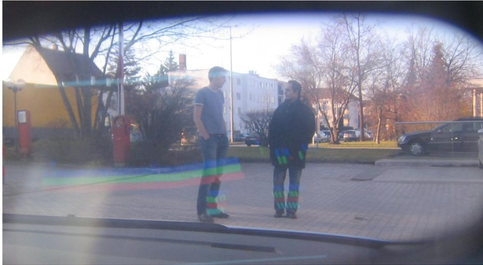
(a) The image shows sensor data from the automotive laser scanner. The persons' legs and the curbstone can be seen superimposed with sensor data.
