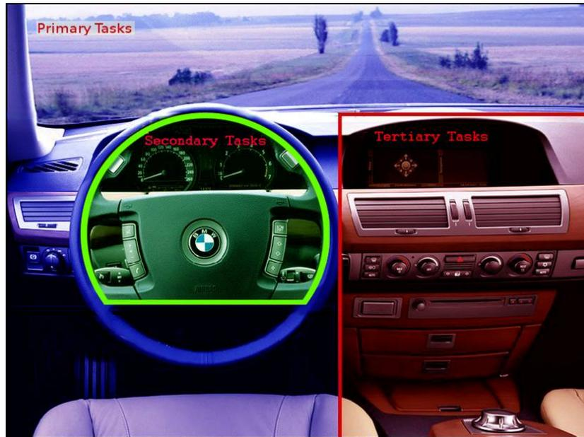
Figure 2.1: Distribution of Primary, Secondary and Tertiary Tasks
