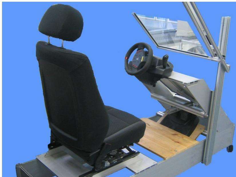
Figure 6.4: The driver's cockpit is built on an aluminum frame and has the same relationships as a common driver's cockpit (distances and sitting height)
