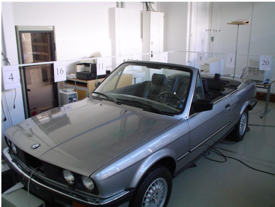
Figure 8.3: Driving Simulator surrounded by Numbered Sheets at Eye Level
