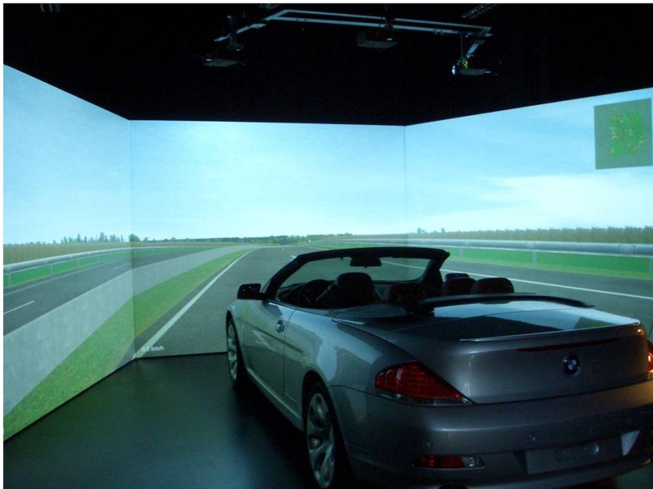
Figure 5.2: The new fixed-base Driving Simulator at the Chair of Ergonomics
