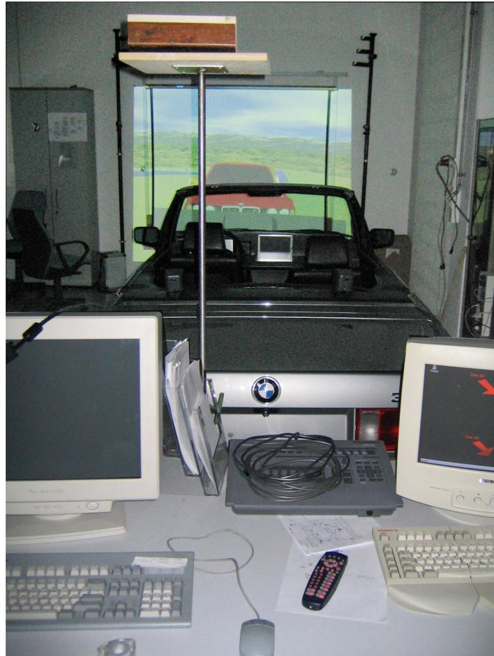
Figure 5.1: The initial Driving Simulator at the Chair of Ergonomics
