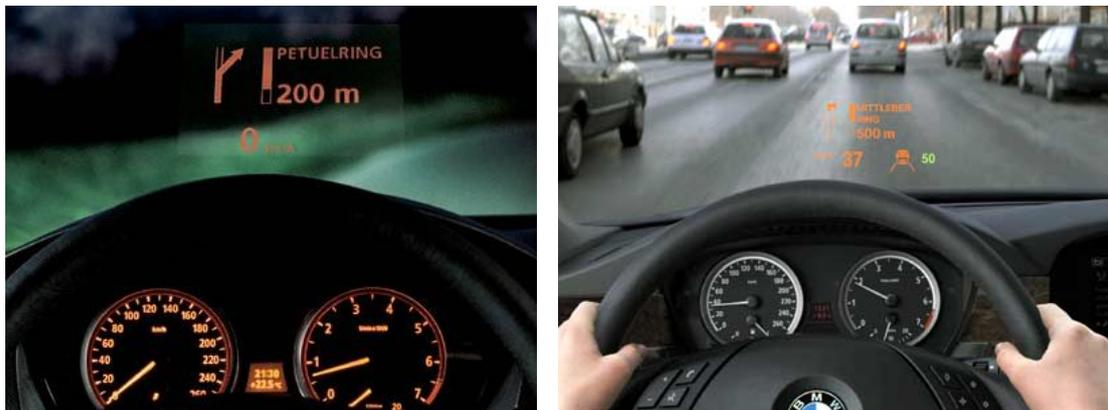
(a) Speed and Navigational Information are shown in most HUDs (b) Some HUDs also show Distance Information. The bright Display also is visible under Daylight Conditions
