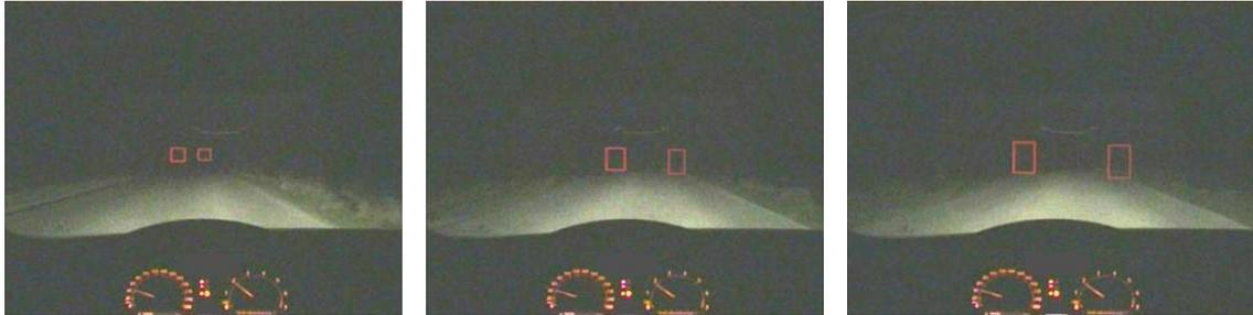
(a) Target objects in 120 m distance; (b) Target objects in 80 m distance; (c) Target objects in 60 m distance; courtesy of [20]
