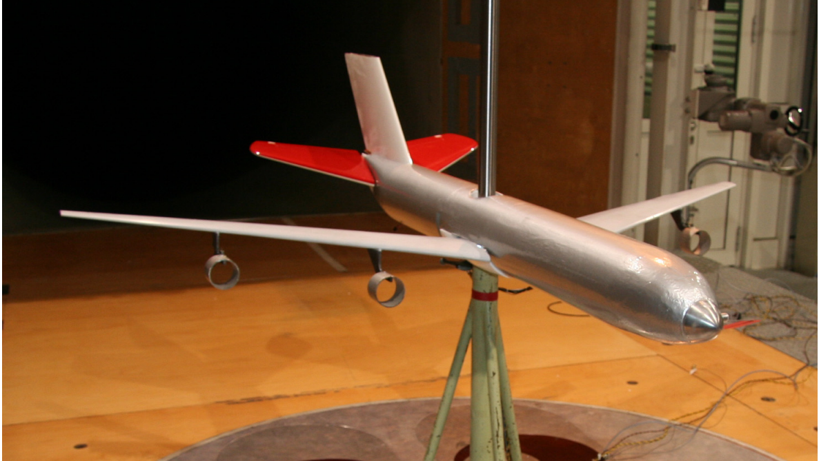
Figure 5-11. The complete elastic aircraft model in the wind tunnel.
