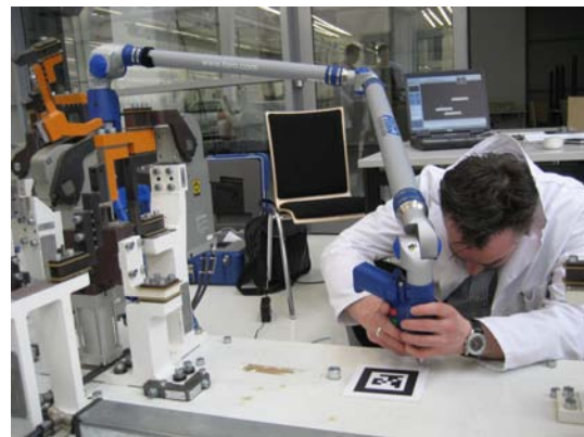
(b) Marker Corner Measurement with the FARO Arm
