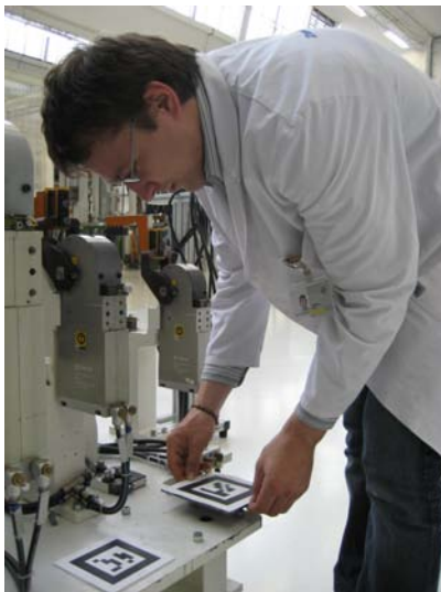
(a) Positioning of Adapter Markers (Source: Volkswagen AG)
