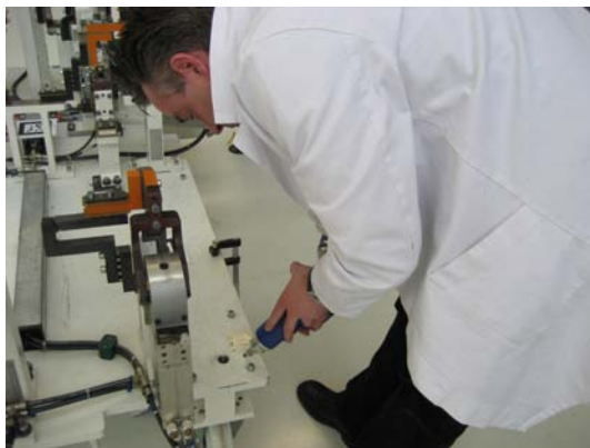
(a) Drill Hole Measurement with the FARO Arm
