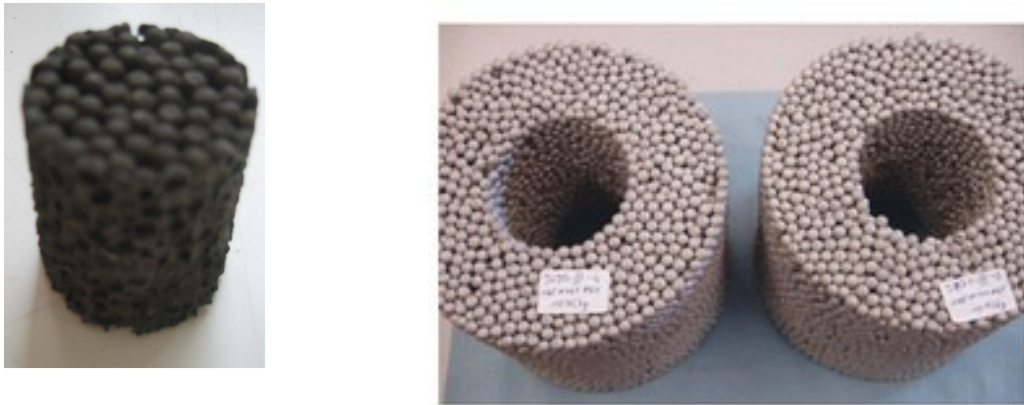
Figure 1: Images of small model structures and the macroscopic structure used in an engine test bench
