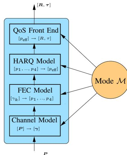
Fig. 1. Components of the System Model
