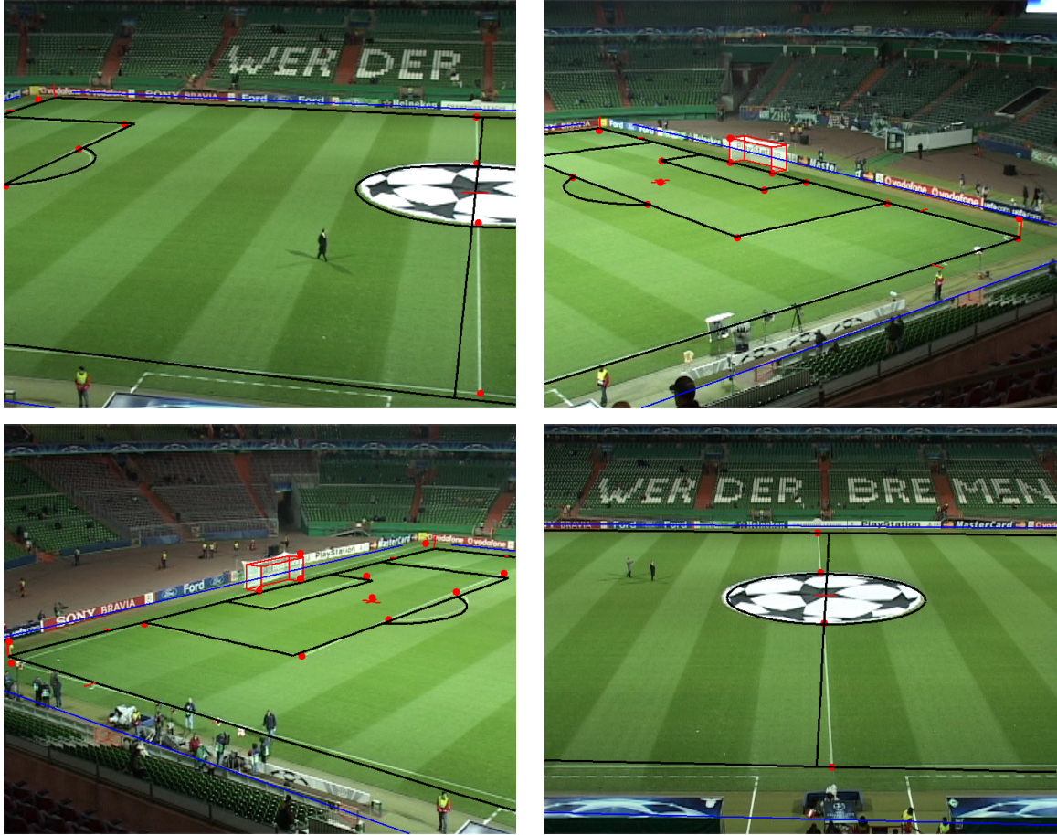
Figure 5.12 Constant Parameter Estimation: Initial estimates determined from point correspondences (red dots)
