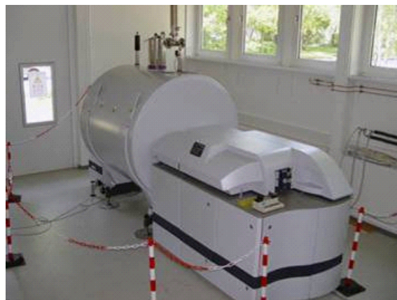
Figure 2.4: 12 Tesla fourier transform ion-cyclotron mass spectrometry (FT-ICR/MS) located at the Institute of Ecological Chemistry, GSF.
