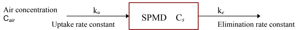
Figure 2-5: Schematic representation of one compartment model for SPMD. C_{air} : compound concentration in air, k_u : uptake rate constant, C_s : compound concentration within the SPMD, k_e : elimination rate constant.
