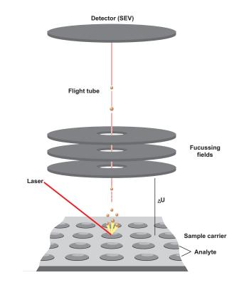
**Figure 3:** Principle of MALDI-TOF. ΔU: accelerating voltage; SEV: secondary electron multiplier
