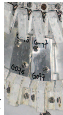
Figure 3.6 (right): Two encapsulated samples, mounted onto the rotary disc of the PNA setup.
