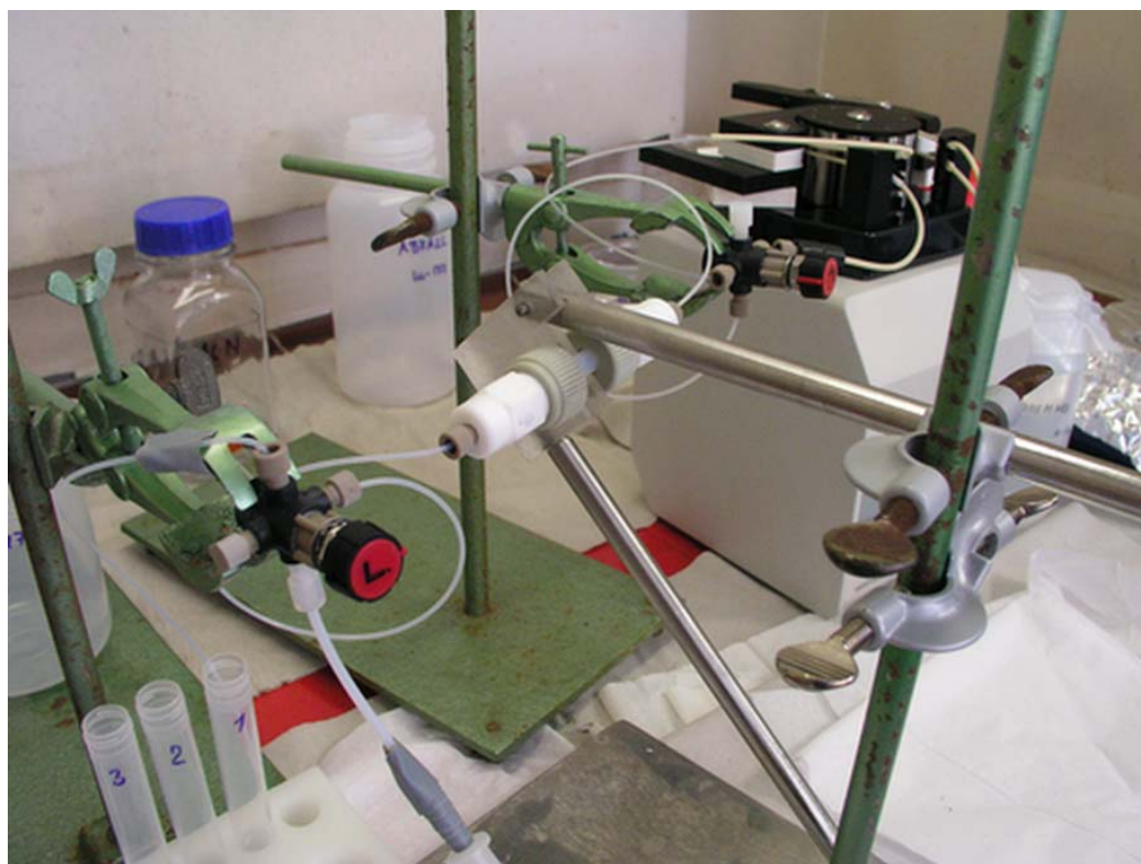
Figure 3.5: Picture of the system for irradiated ampoule breaking. Detailed description in text.
