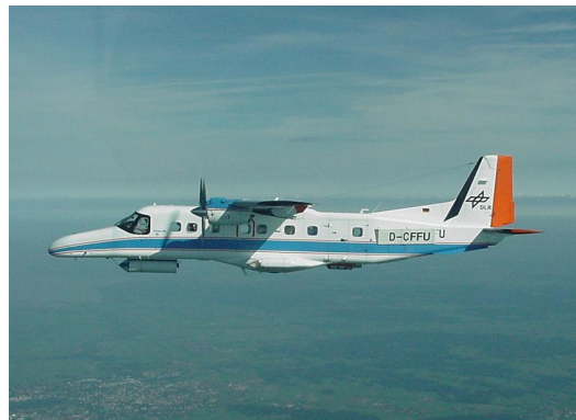
Fig. 3-4 The airborne 'Experimental-SAR' system of DLR (E-SAR): system parameters and DO-228 carrier platform
