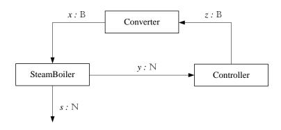
Figure 2.3.: Architecture of the Steam Boiler System
