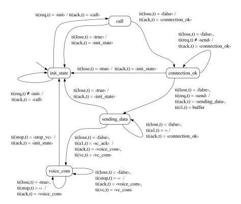
Figure 4.1.: Timed state transition diagram for the component Sample
