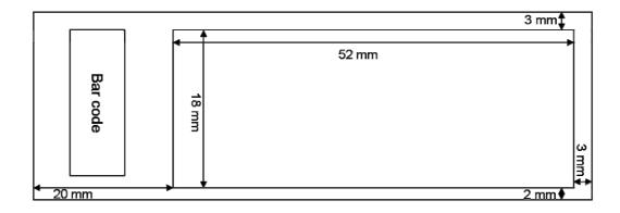
Figure 7. SCMV array layout. Spotted area of the SCMV array: 52 x 18 mm
