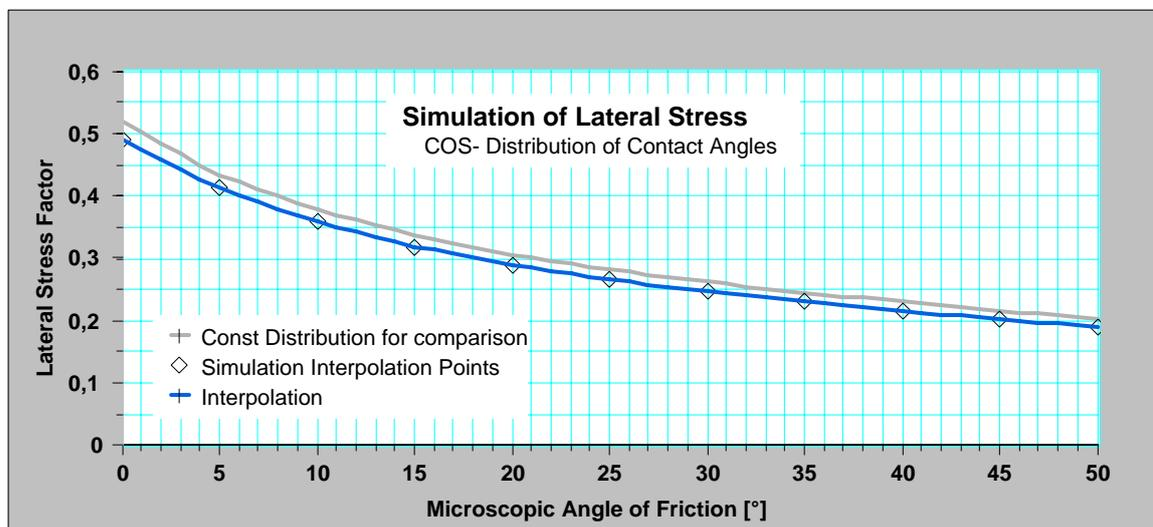
FIG. 102. Averaged lateral stress factor, using a COS distribution (File: NumSimulations.123)
