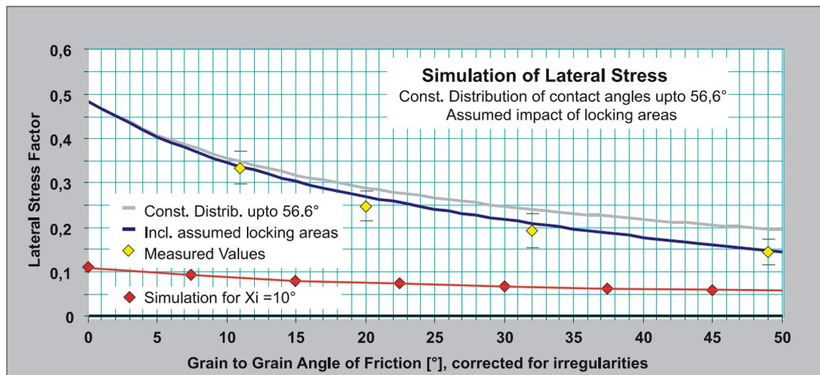
FIG. 111. Simulation of very straight force chains, lateral stress (File: NumSimulation.123)
