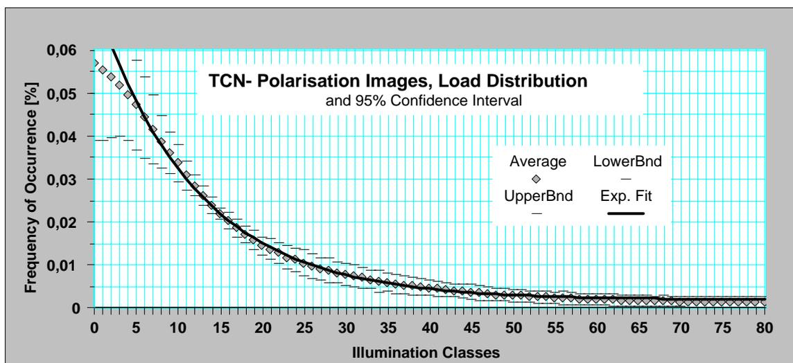
FIG. 153. Typical analysis of light intensities of several images, obtained from Polyester cylinders (File: TCN-Distrib.123)
