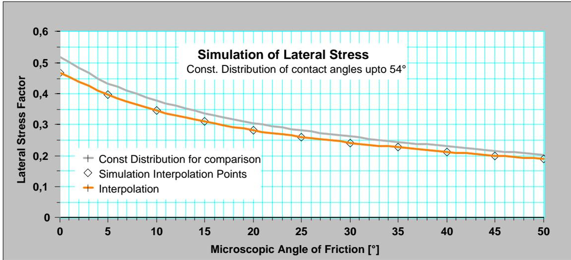
FIG. 103. Lateral Stress Factor using a Const. Distribution limited to 54° (File: NumSimulation.123)
