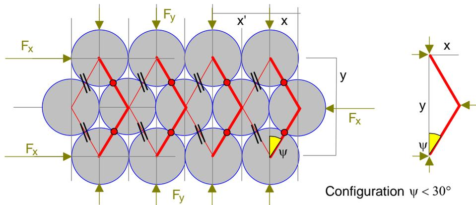
FIG. 116. Arrangements of cylinders, where symmetry is broken
