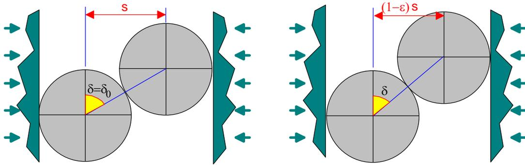
FIG. 67. Deriving  $\delta$  as a function of the deformation  $\epsilon$
