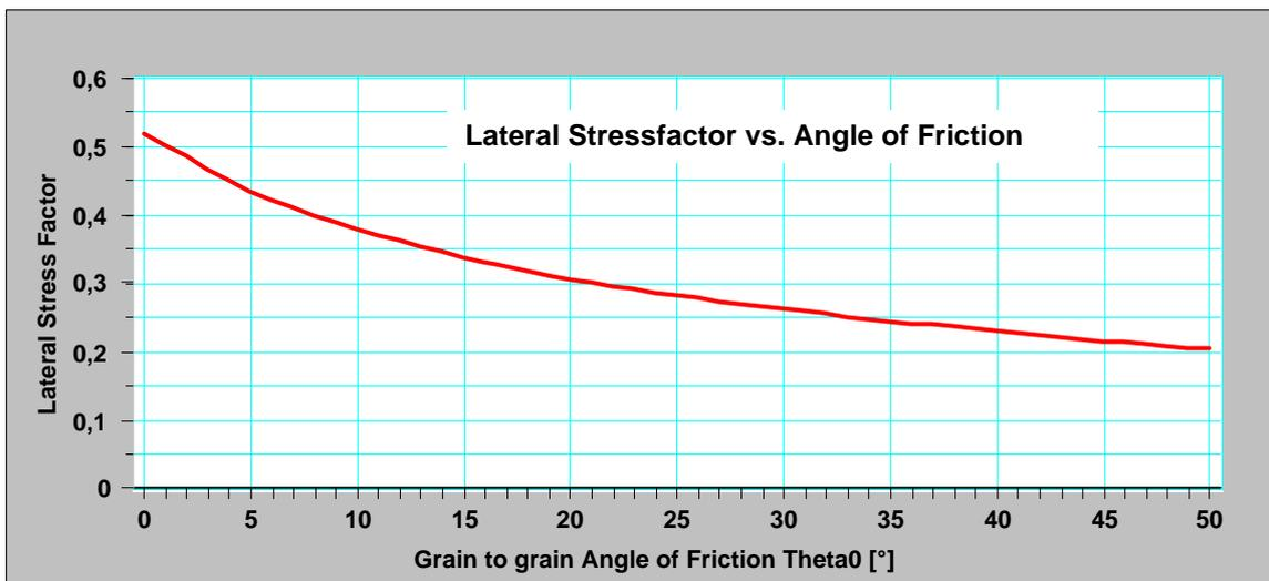
FIG. 125. Numerically obtained lateral stress factor for LLO systems (File: NumSimulation ReachOut.123)
