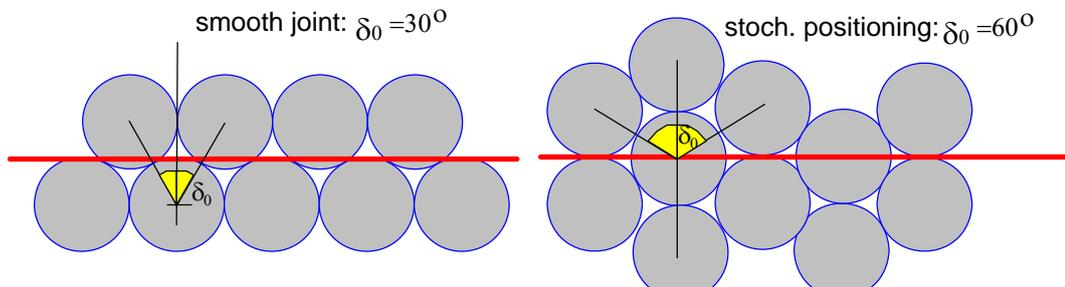
FIG. 66. Dependence of  $\delta_0$  on the smoothness of the shear joint
