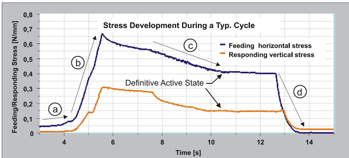
FIG. 21. Typical stress development during deformation cycle (File: MeasurementCycle UCT25.123)
