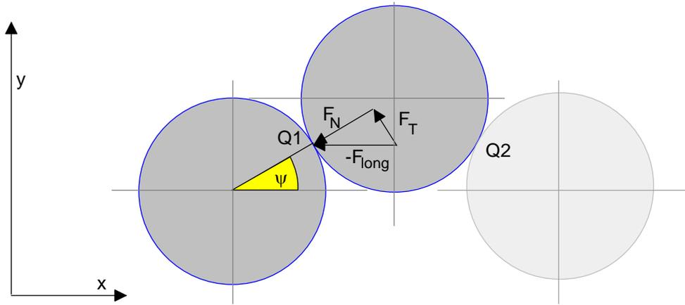
FIG. 80. Criterion of Gliding in preliminary model
