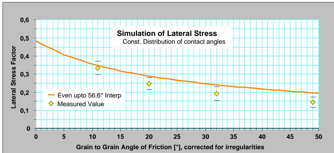
FIG. 106. Averaged lateral stress factor in comparison to measured values (File: NumSimulation.123)
