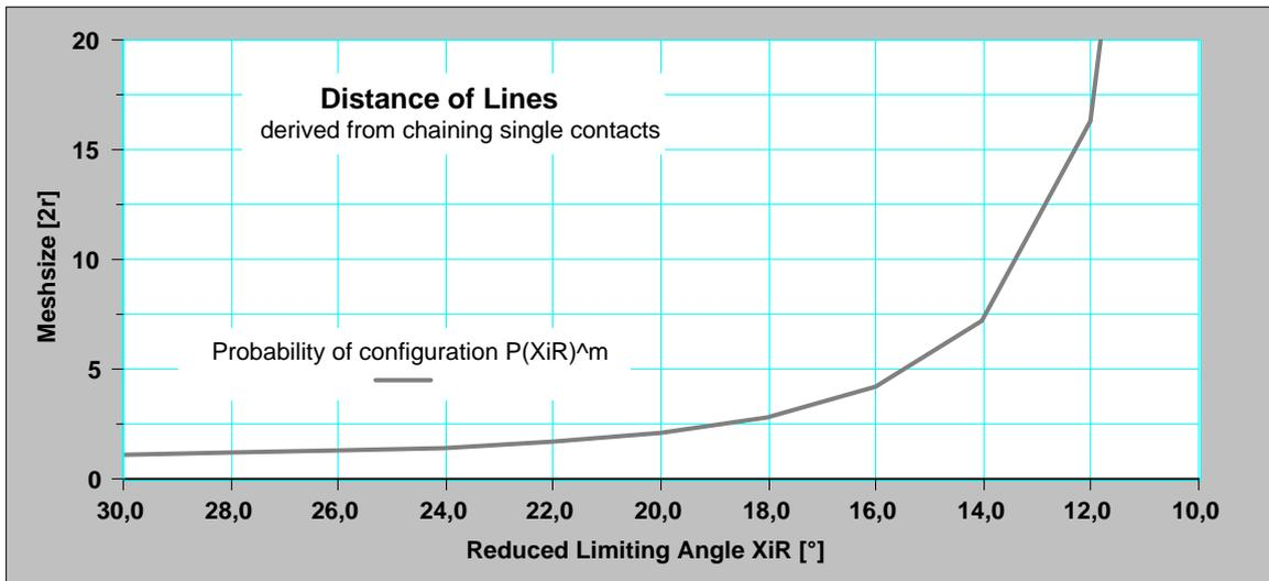
FIG. 150. Required distance of force chains resulting from chaining single contacts (File: StifferLines.123)
