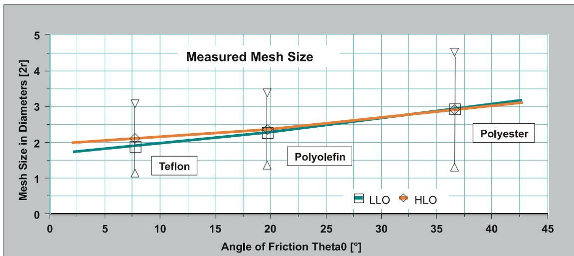
FIG. 47. Experimentally obtained av. meshsize (File: MeshSizeInterpr.123)
