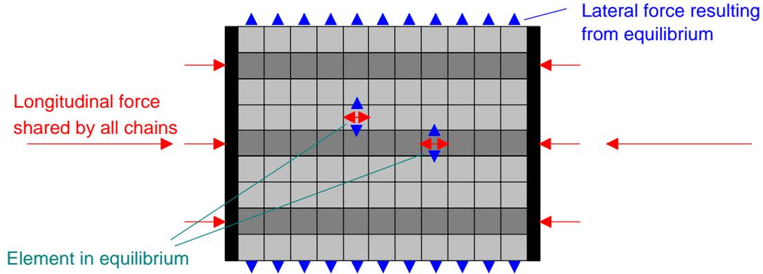
FIG. 143. Equilibrium in a granular system, where some chains bear most of the longitudinal stress
