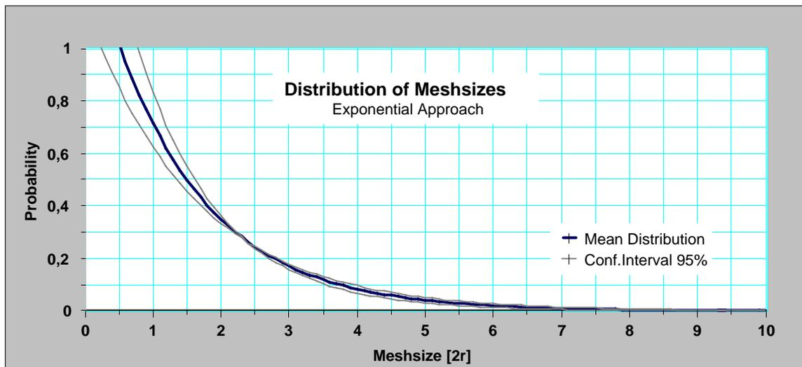
FIG. 152. Predicted exponential distribution of mesh sizes resp. chain lengths (File: DistribOf MeshSize.123)
