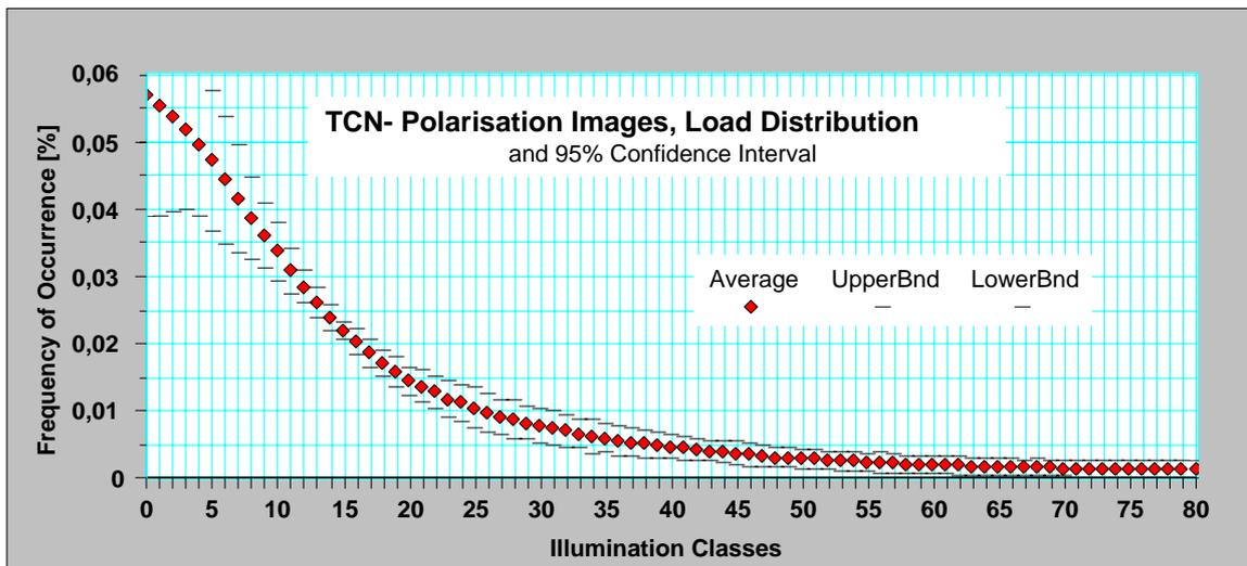
FIG. 44. Typical analysis of light intensities of several images, obtained from Polyester cylinders (File: TCN-Distrib.123)
