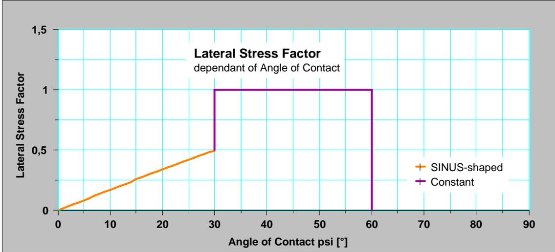
FIG. 117. Lateral Stress Factor for special arrangements of cylinders, where  $\vartheta_0 = 0$  (File: ExtremeCasesSymm60°.123)
