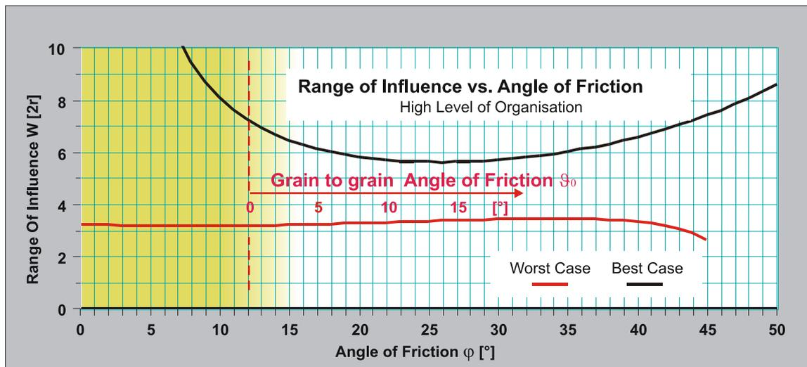
FIG. 128. Range of influence, limited by friction in highly organised systems (File: NumComputation ReachOutTwoCases.123)
