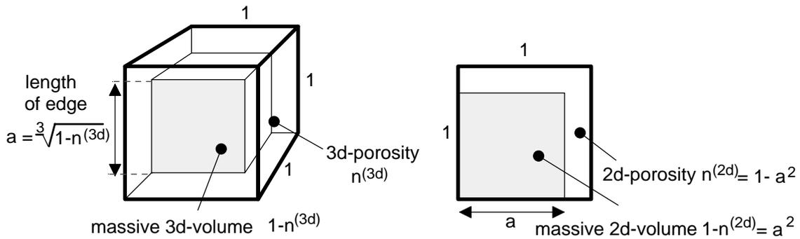
FIG. 6. Estimation of 2d-porosity from 3d measurements
