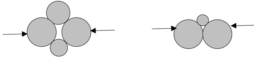
FIG. 107. Some configurations of higher order causing 'Locking Areas' inducing no Lateral Stress
