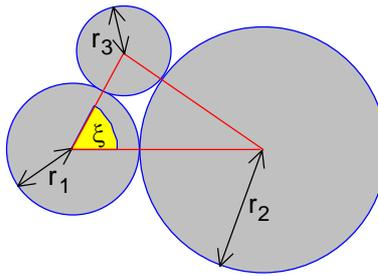
FIG. 88. Possible maximum angles of contact in polydisperse media
