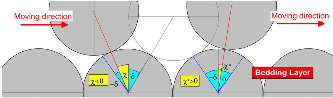
FIG. 63. Geometrical situation in the sliding joint (Clockwise oriented angles are positive).
