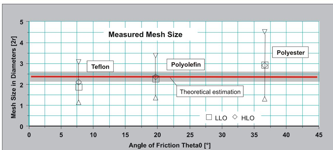
FIG. 154. Comparison of theoretical meshsizes vs. experimentally obtained values (File: MeshSizeInterpr.123)
