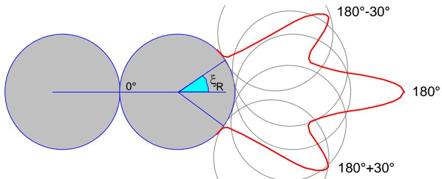
FIG. 141. Typical distribution of contact angles
