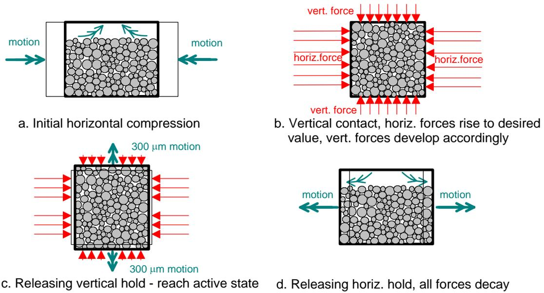
FIG. 20. Schematic view of measurement cycle to achieve an active state. **Bold** double arrows indicate motion while **light** arrows are forces
