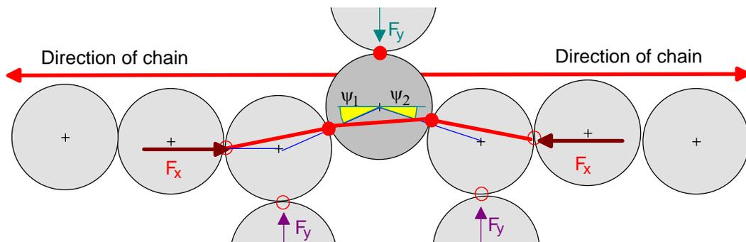
FIG. 86. Single cylinder within a chain, three dominating contacts
