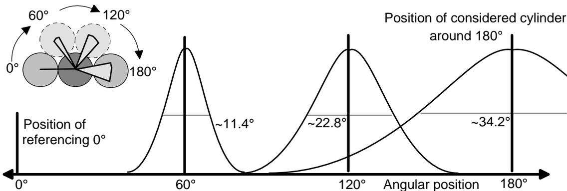
FIG. 137. Extent of contact angle distribution for the set of cylinders used in this paper
