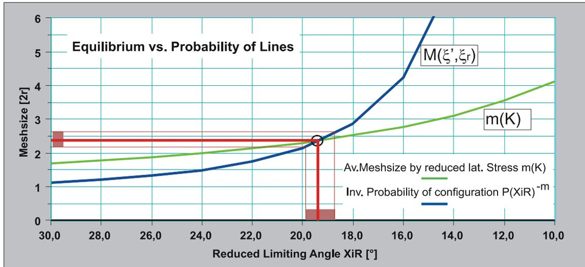
FIG. 151. Required distance of force chains, both approaches (File: StifferLines.123)
