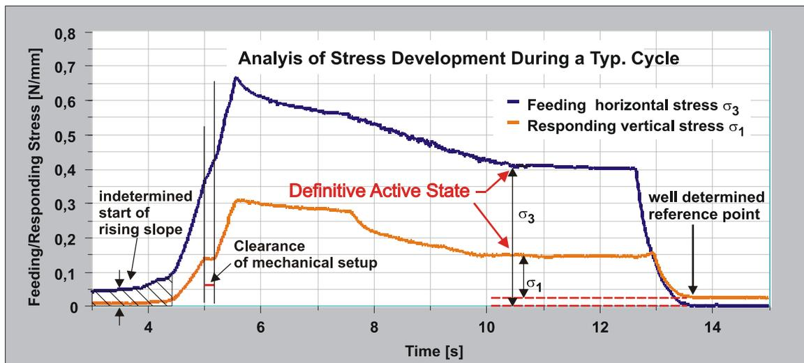
FIG. 23. Typ. Stress development and possible reference point (File: Reference for MeasurementCycle UCT25.123)
