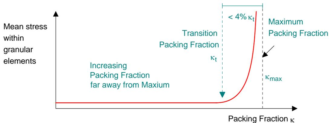
FIG. 56. Qualitatively rising mean stress with increasing packing fraction
