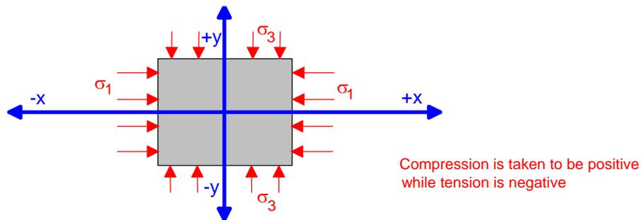
FIG. 19. Orientation and coordinate system used in this paper
