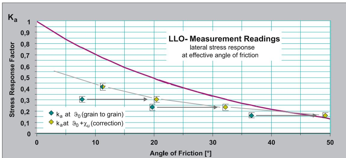
FIG. 77. Correction to measured values due to surface unevenness (File: Readings.123)
