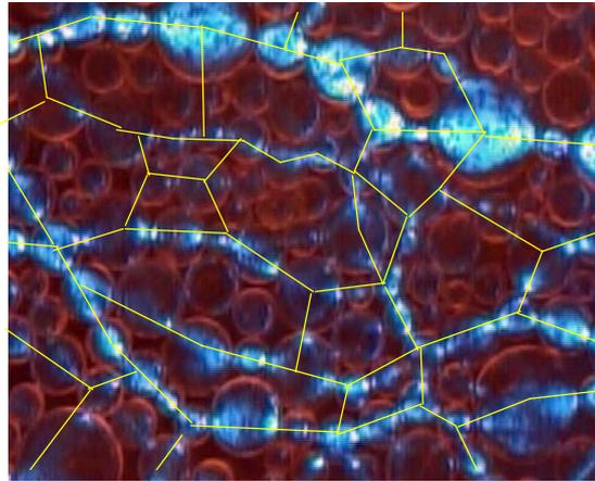
FIG. 119. Picture from the polariscope, displaying the building of a force network
