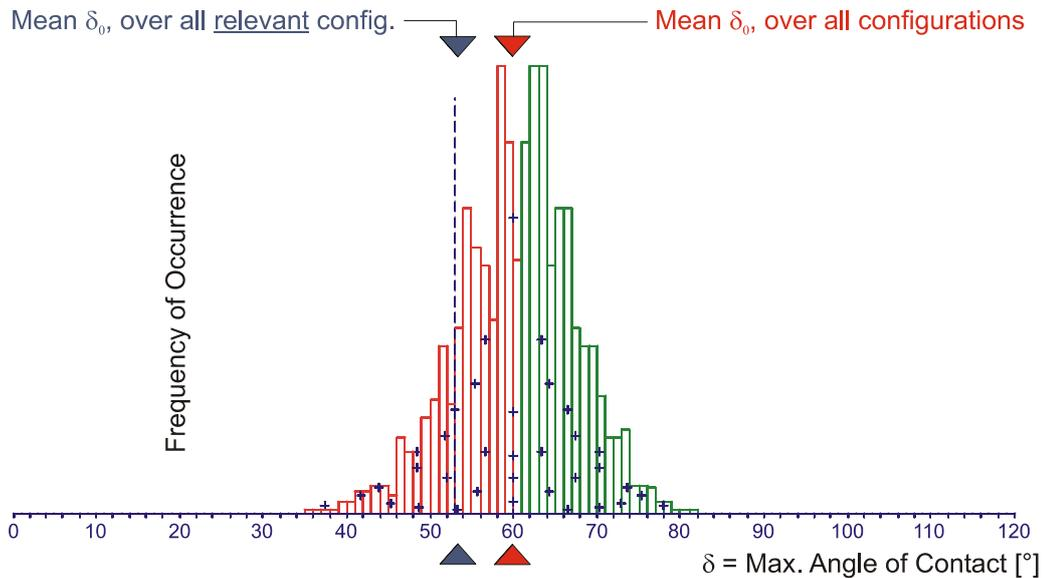
FIG. 69. Numerically obtained distribution of the max. Angle of Contact for the set of cylinders used here.
