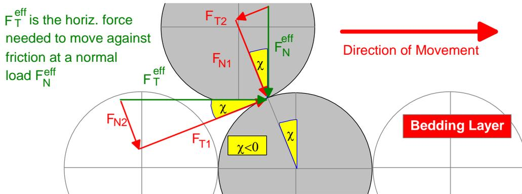
FIG. 64. Composition of forces within a sliding joint
