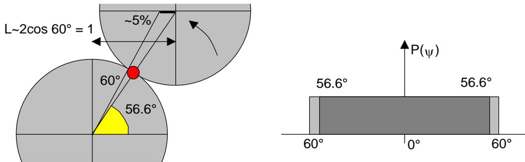
FIG. 104. Limiting the range of contact angles to  $56.6^\circ$  by a deformation of  $\sim 5\%$
