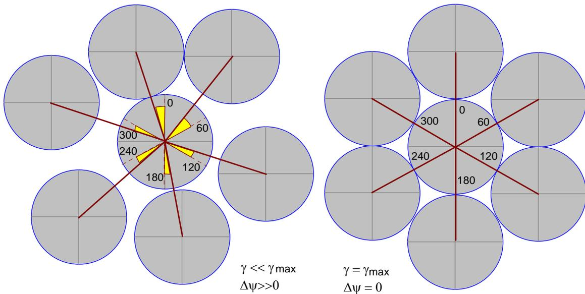
FIG. 134. Reduced degree of freedom in dependency of packing fraction (monosized cylinders)
