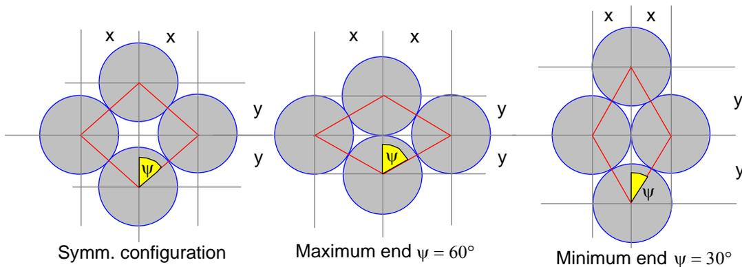
FIG. 115. Symmetrical arrangement of equally sized cylinders
