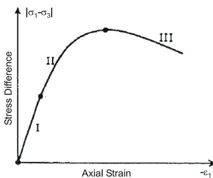
FIG. 1. Typical dependency of shear stress vs. strain.
