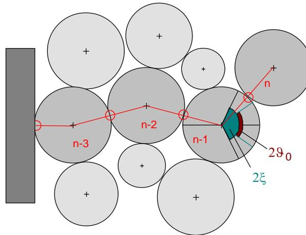
FIG. 130. Model of force chain, defined by fixed cylinders, where the first non rolling contact terminates the chain.
