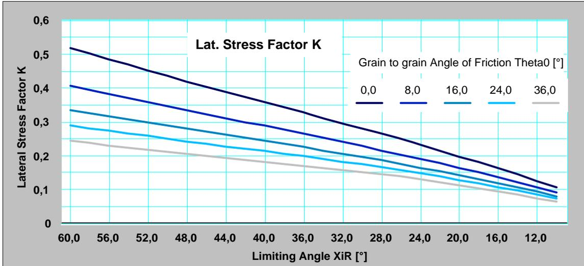
FIG. 146. Lateral stress factor under limited range of contact angles (File: StifferLines.123)
