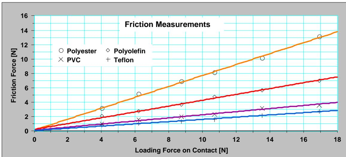
FIG. 18. Friction forces vs. normal load, experimentally obtained from different surface coatings (File: FrictionComplete.123)
