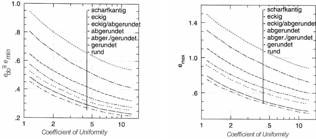
FIG. 5. Minimum and maximum void ratio dependent on uniformity and shape of granules (according to [30])
