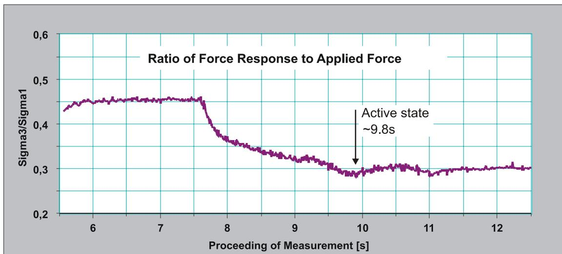
FIG. 24. Confirmation of active state as the minimum of the force ratio (File: MeasurementCycle Min UCT25.123)
