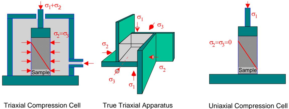
FIG. 3. Experiments allowing for free development of a shear joint
