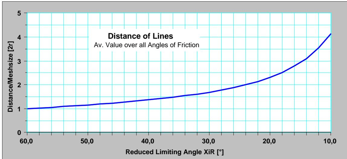
FIG. 148. Required distance of force chains resulting from limited range of contact angles (File: StifferLines.123)
