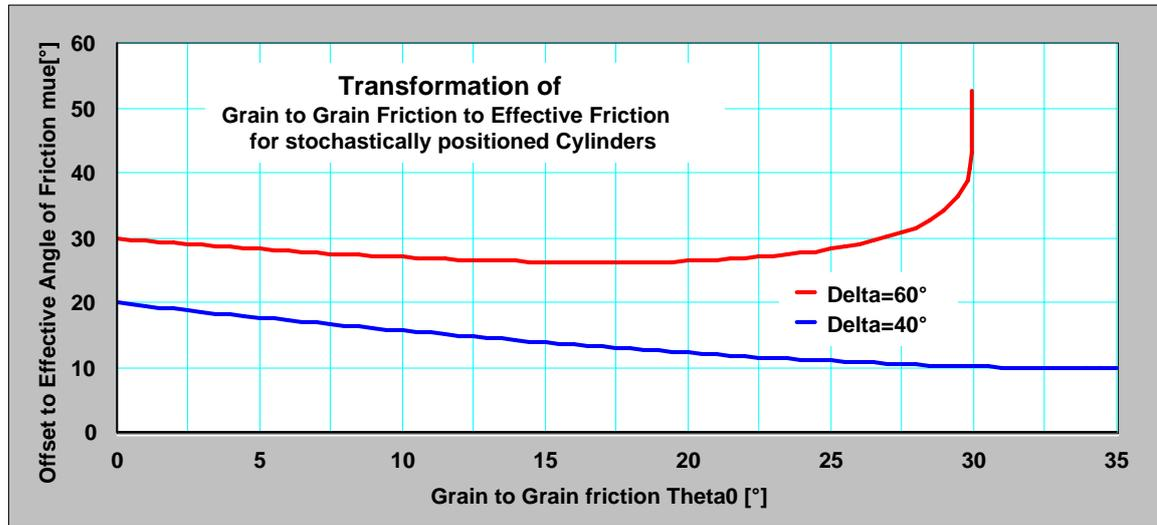
FIG. 110. Transformation of Grain to Grain Friction  $\Theta_{00}$  to effective friction  $\mu_{00}^{eff}$  for stochastically positioned cylinders
