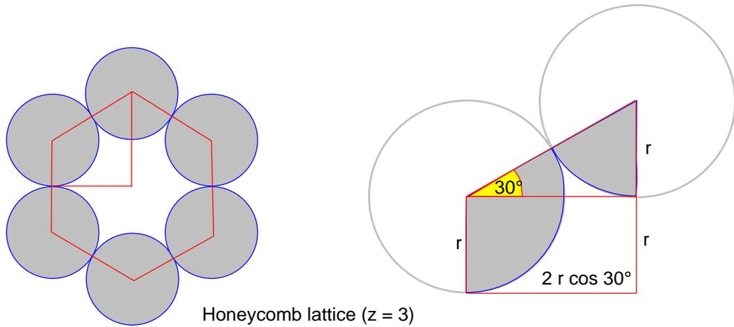
FIG. 49. Theoretical porosity of a honey comb lattice
