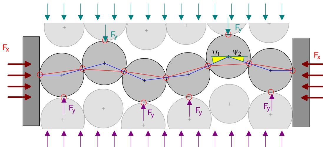
FIG. 84. Model of parallel chains of cylinders bearing the longitudinal force
