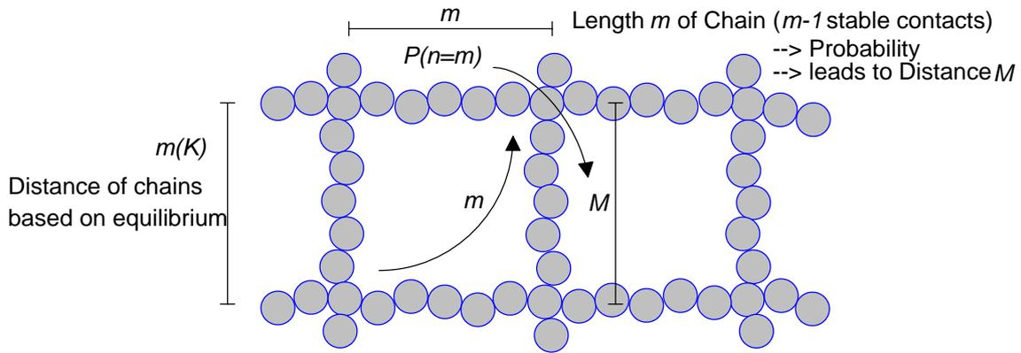
FIG. 149. Correlation of longitudinal and transversal chain distances and -lengths
