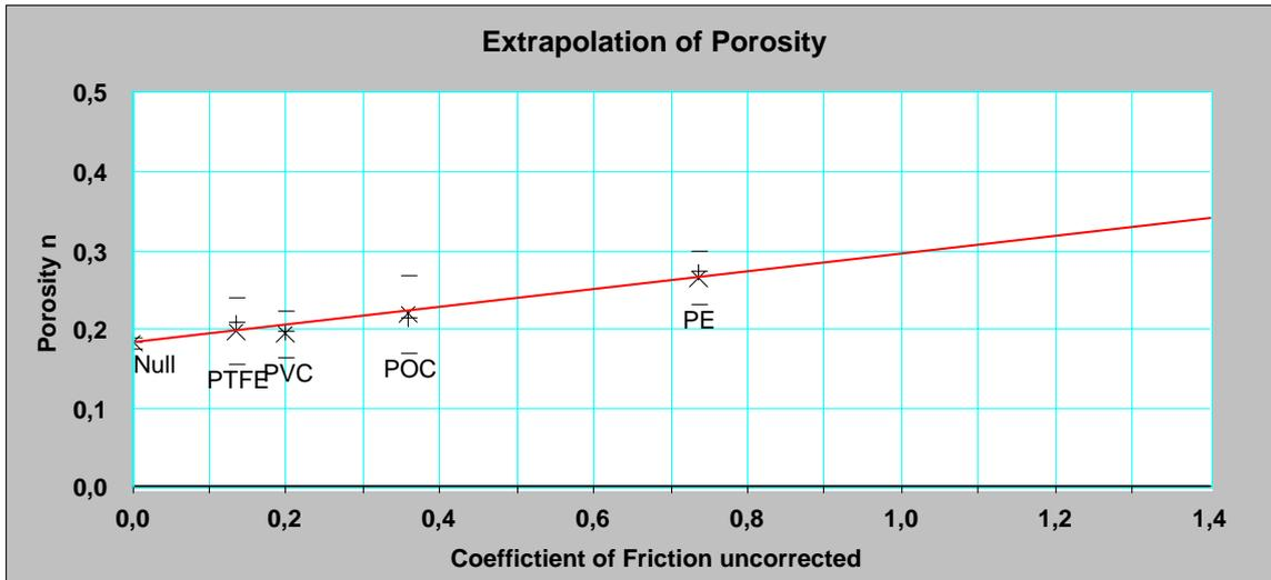
FIG. 54. Linear interpolation for measured porosity values (File: InterpolationOfPackingFraction.123)
