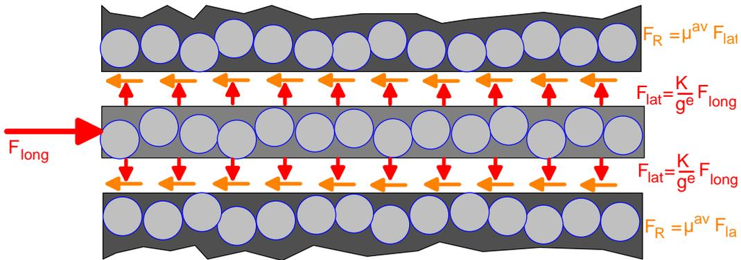
FIG. 124. A single force chain limited in length of effectiveness by friction  $\mu^{av}$  versus environment
