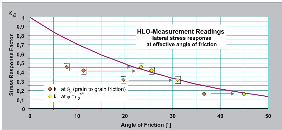
FIG. 71. Measured values, transformed using  $\delta(\epsilon)$  instead of  $\delta_0$  correspond to the Rankine approach (File: Readings.123)
