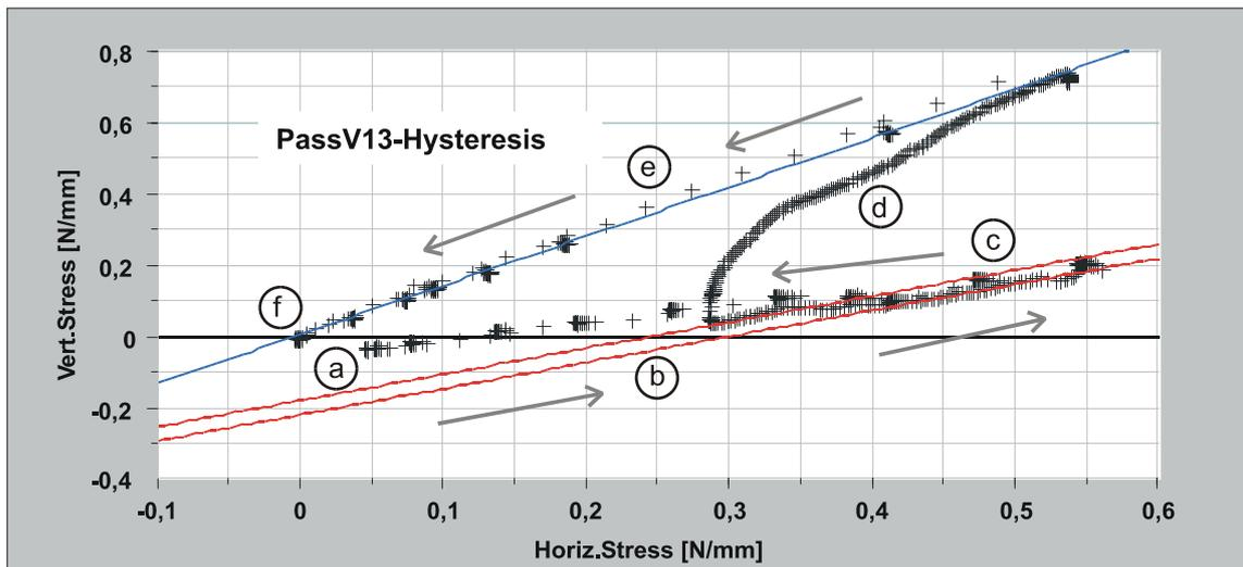
FIG. 34. Exemplary measurement II results confirming the achievement of an active state (File: PassV13 Diagram Disp.123)
