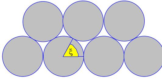
FIG. 87. Constant maximum angle of contact in monodisperse media
