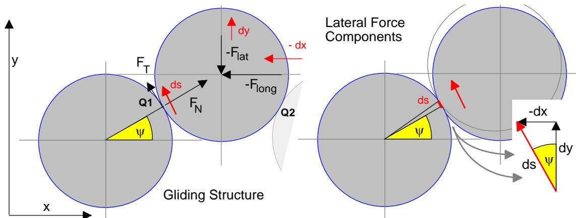
FIG. 81. Redirection of forces in preliminary model
