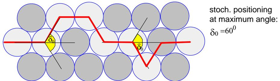
FIG. 74. Maximum Angle of Contact  $\delta_0$  in a stochastically positioned set of cylinders
