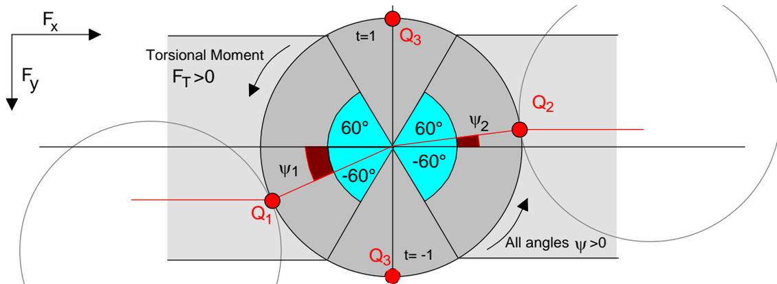
FIG. 90. Definition of possible contacts for an isolated cylinder
