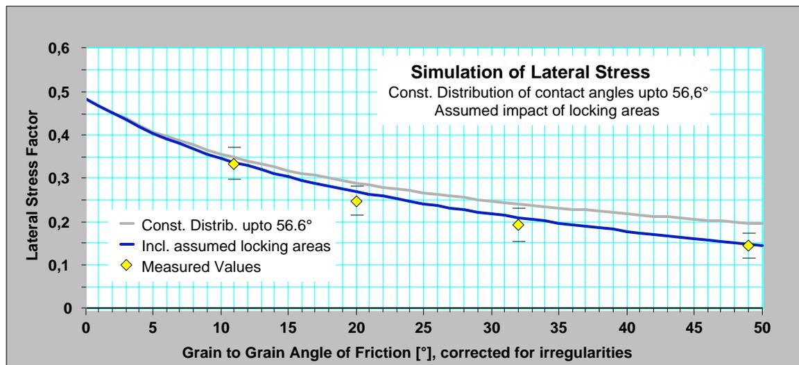
FIG. 108. Simulation results with assumed locking areas in comparison to measured values (File: NumSimulation.123)
