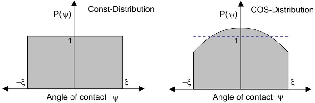
FIG. 100. Constant Distribution of contact angles vs. COS Distribution
