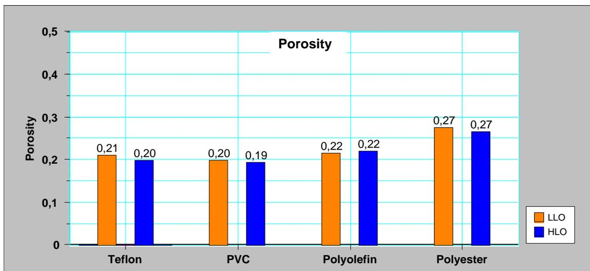
FIG. 52. Measured porosity values (File: PackingDensity.123)
