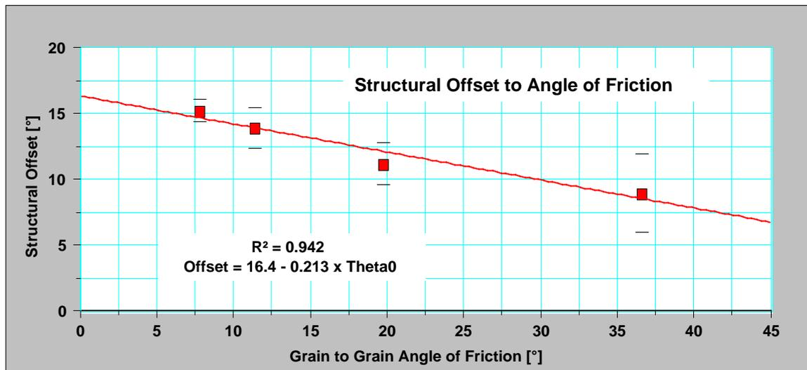
FIG. 72. Linear fitting approach for the structural offset to the Rankine model (File:StructuralOffsetTCFit.123)
