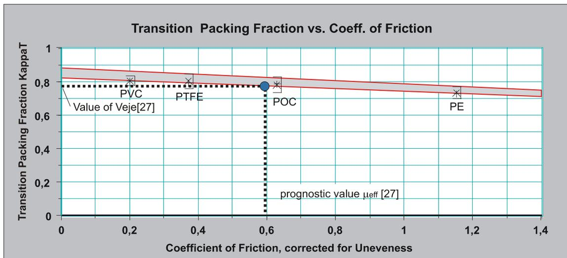
FIG. 59. Estimation of development of packing fraction (File:CriticalPackingFraction.123)
