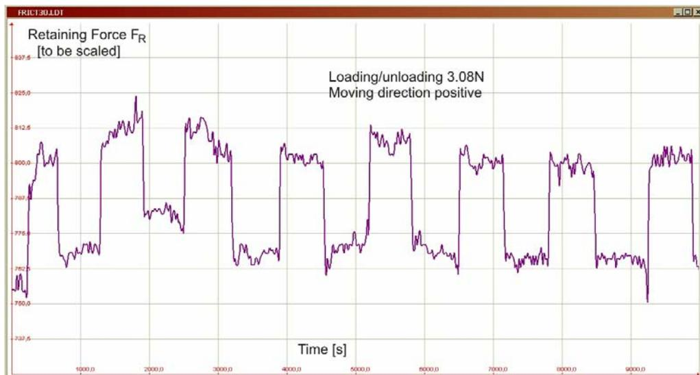
FIG. 17. Typical plot of friction force vs. measurement time during load steps (File:FrictionDemo.JPG)
