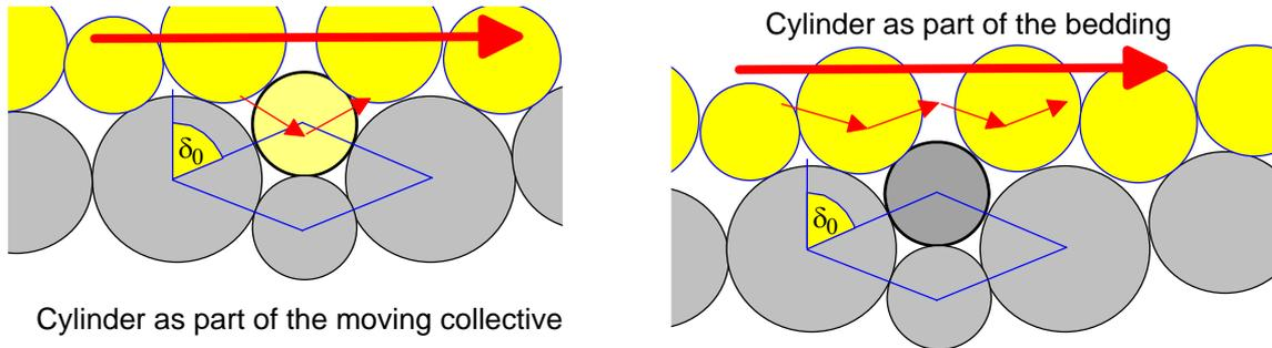
FIG. 70. Changeover of a single cylinder in the sliding joint from the moving block to the bedding
