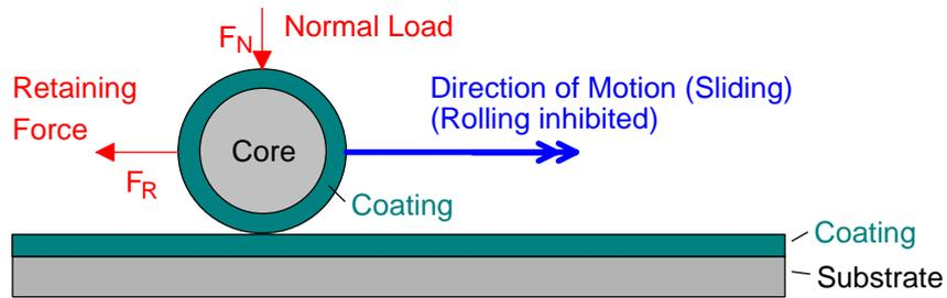
FIG. 16. Schematic view of the experimental setup used to measure friction parameters
