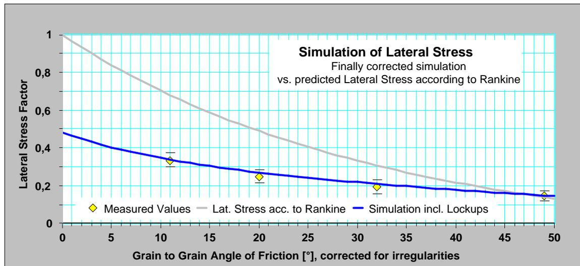
FIG. 109. Simulation results with assumed locking areas in comparison the Rankine prediction (File: NumSimulation.123)
