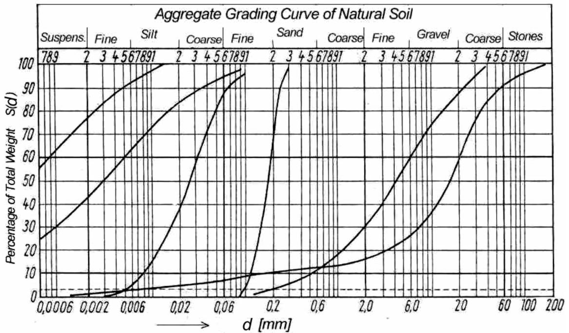
FIG. 7. Aggregate Grading Curve of Natural Soil (according to [57])
