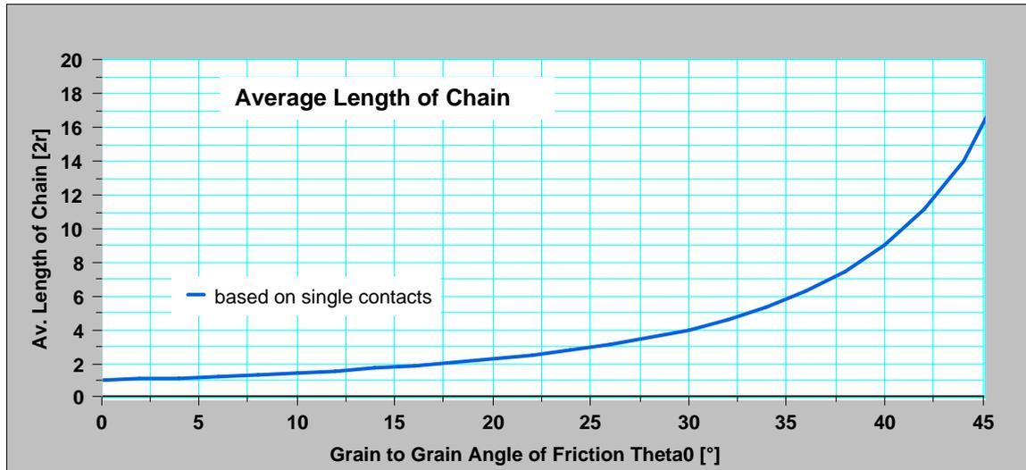
FIG. 131. Av. length of chains, derived from 'rolling vs. gliding' criterion (File: LineLengths.123)
