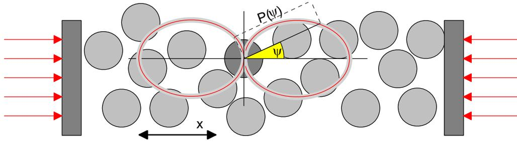
FIG. 120. Schematic view of the probability of generating further contacts (neglecting own weight)
