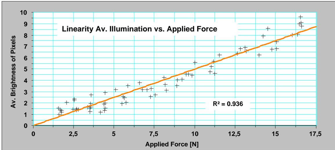
FIG. 41. Confirmation of a linear dependency of illumination values vs. the applied forces (File: Force-Illum-Dep.123)
