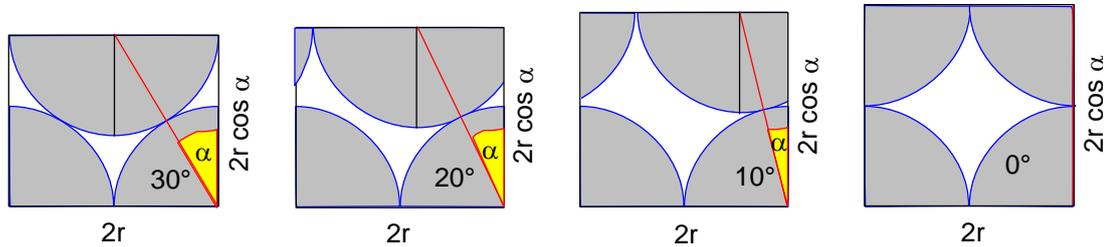
FIG. 51. Estimation of packing fraction of a random close packing
