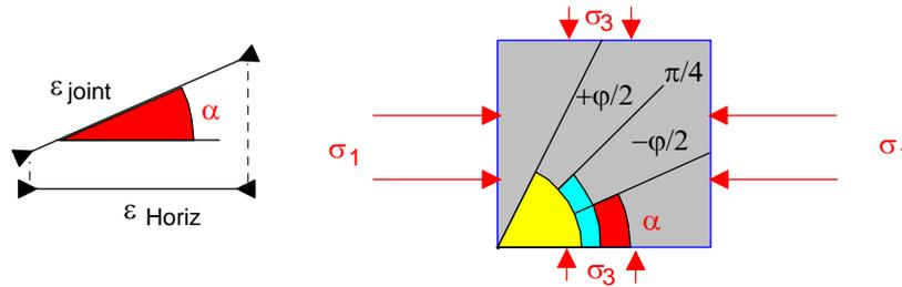
FIG. 68. Transforming horizontal compression to angular compression
