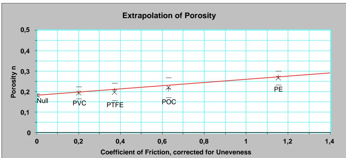
FIG. 55. Linear interpolation for measured porosity values, corrected for irregularities (File: InterpolationOfPackingFraction.123)
