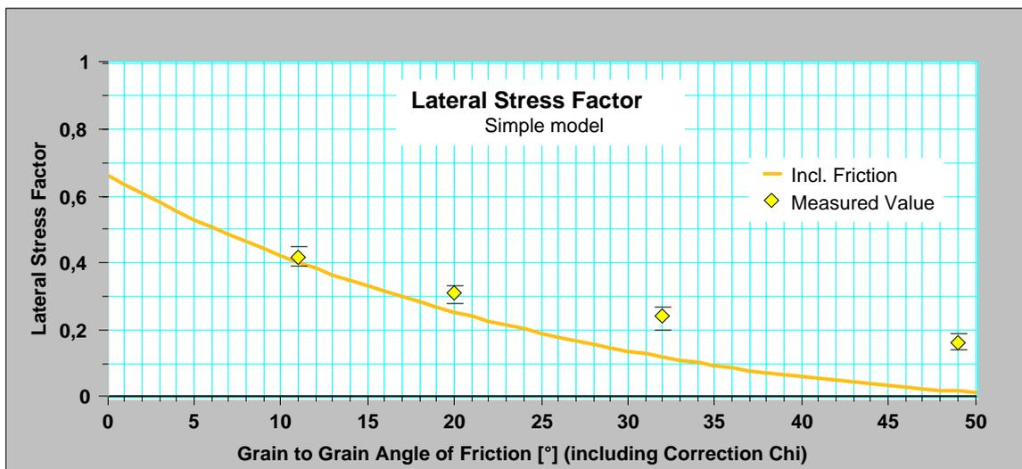
FIG. 83. LLO-Measurement of Lateral Stress Factor and result of highly simplified model (File: SimplifiedModelLLO.123)
