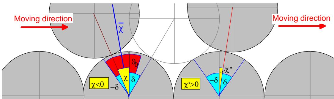
FIG. 126. Effective friction in a sliding joint, represented by average angle  $\bar{\chi}$
