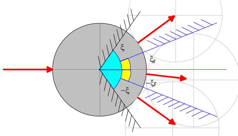
FIG. 133. Definition of a reduced range for contact angles
