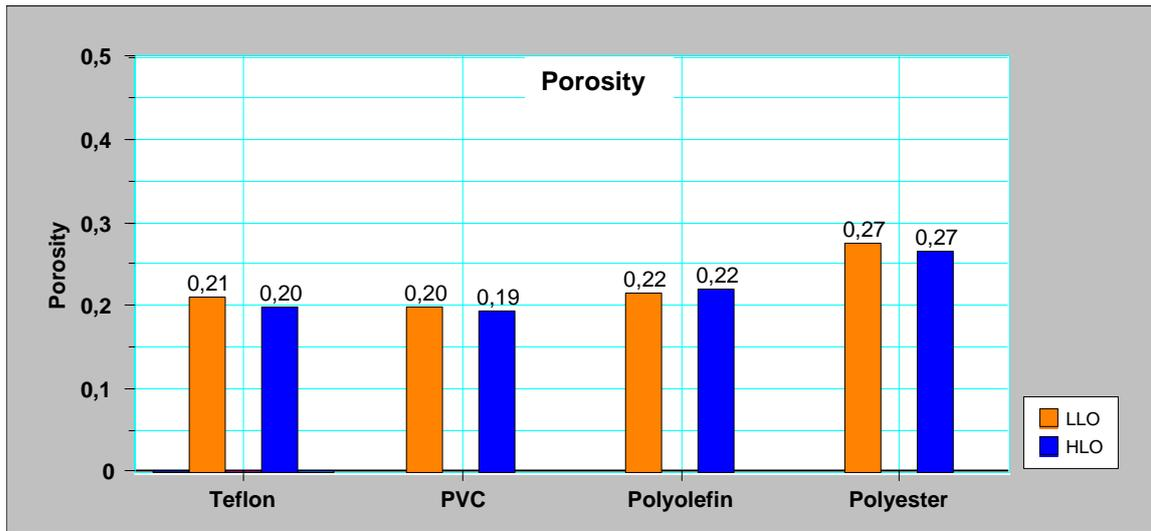
FIG. 37. Measured porosity values (File: PackingDensity.123)
