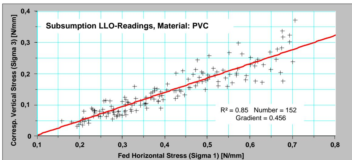
FIG. 26. Exemplary set of measured values: Horiz. stress vs. responding vert. stress (File: Subsumption UCV.123)
