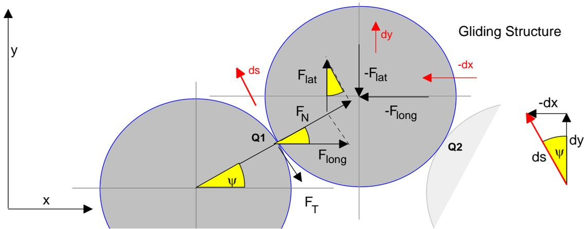
FIG. 82. Retaining friction forces in preliminary model
