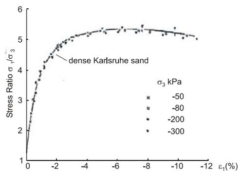
FIG. 2. Measured dependency of shear stress vs. strain
