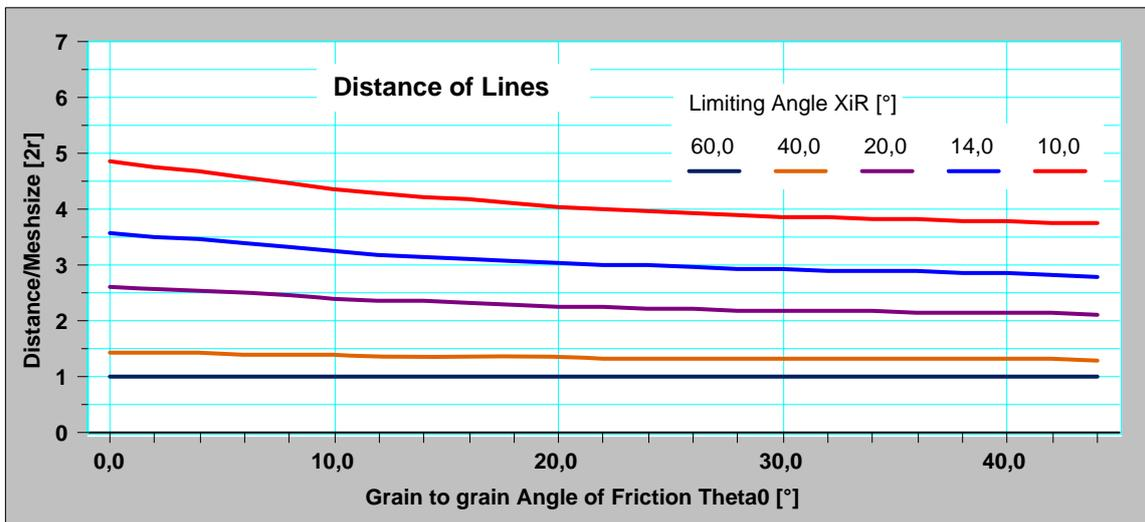
FIG. 147. Required distance of force chains resulting from limited range of contact angles (File: StifferLines.123)
