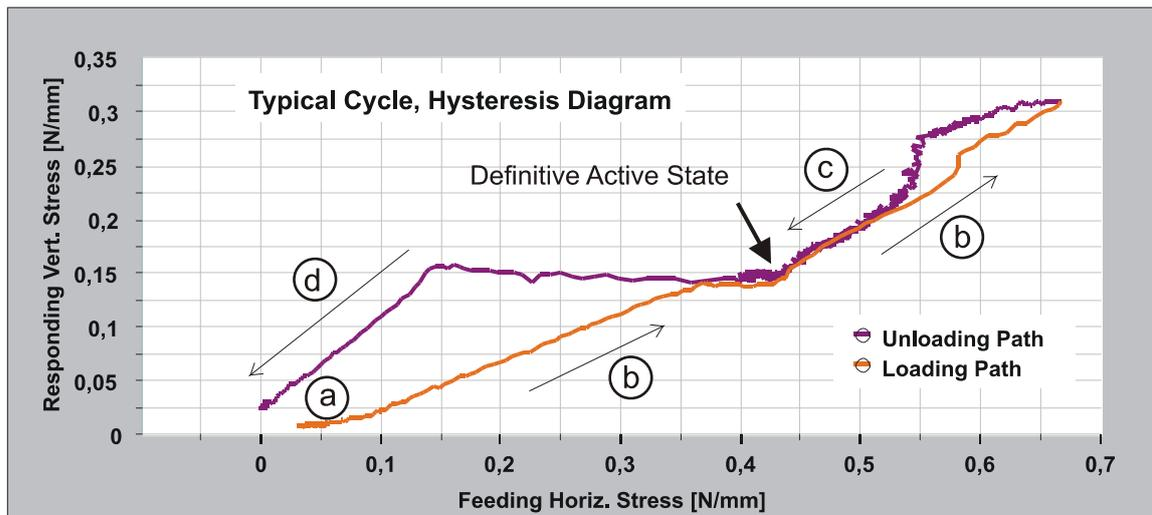
FIG. 22. Hysteresis diagram of typical deformation cycle (File: MeasurementCycle UCT25.123)
