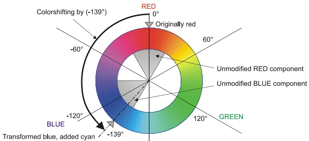
FIG. 39. Consequences of the colorshifting process applied to polariscope images (File: ColorcircleFinal.cdr)
