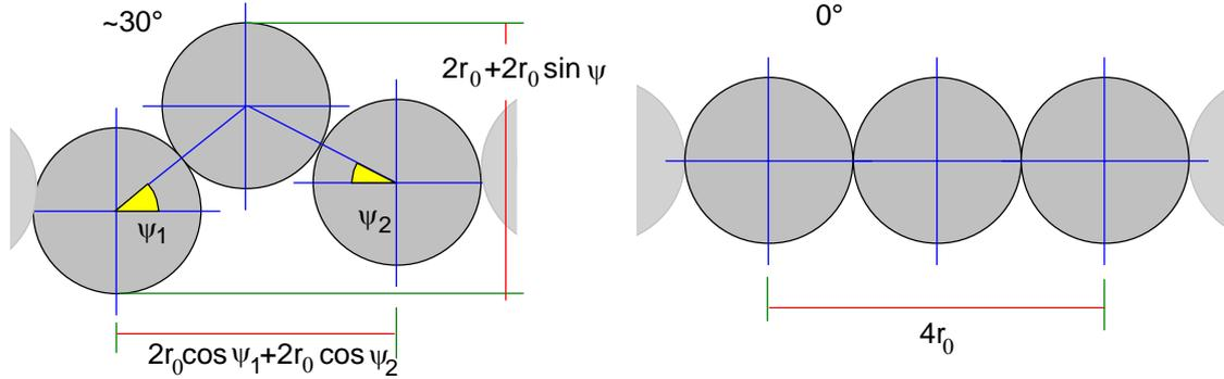
FIG. 97. Geometric extent of 'basic cell' depending on angles of contact  $\psi$
