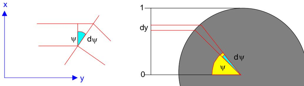
FIG. 96. Linear deformation, leading to a COS distribution of contact angles
