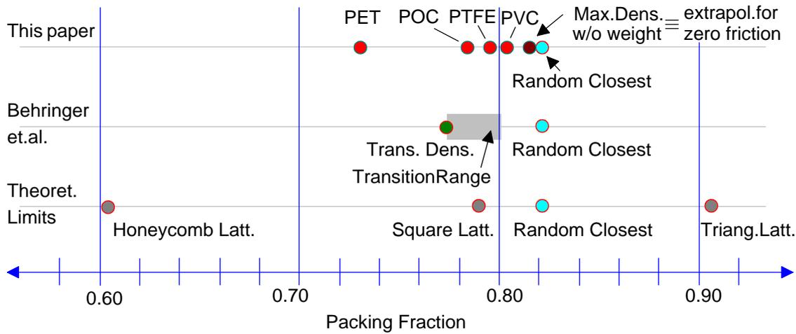
FIG. 57. Comparison of packing fraction values obtained by different sources
