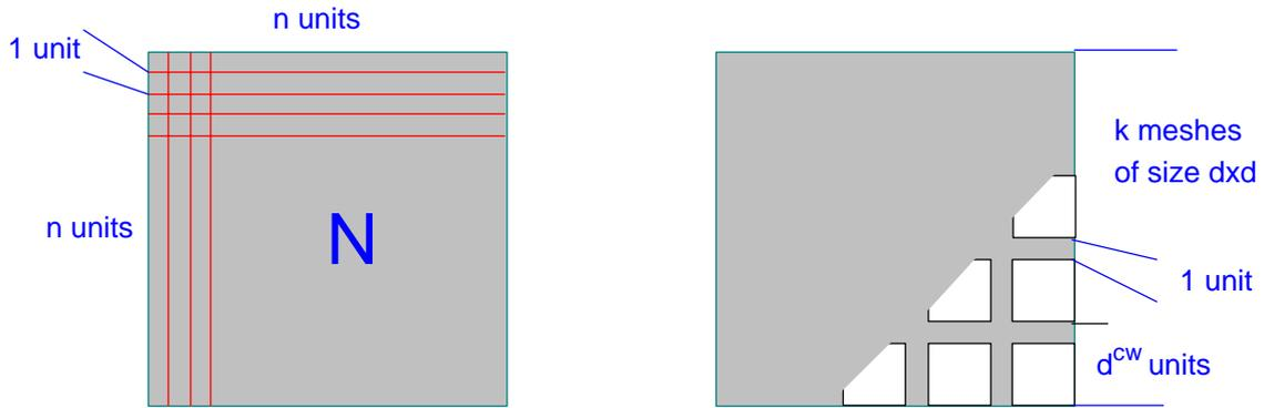
FIG. 45. Geometrical aspects of a network with meshlines of finite width
