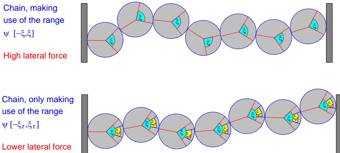
FIG. 144. Reduction of lateral stress by limiting the range of possible contact angles
