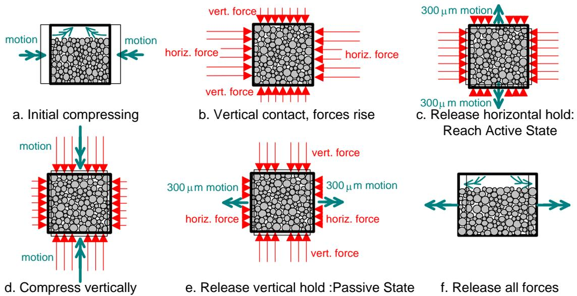
FIG. 32. Schematic view of extended measurement cycle. Bold double arrows indicate motion while light arrows are forces
