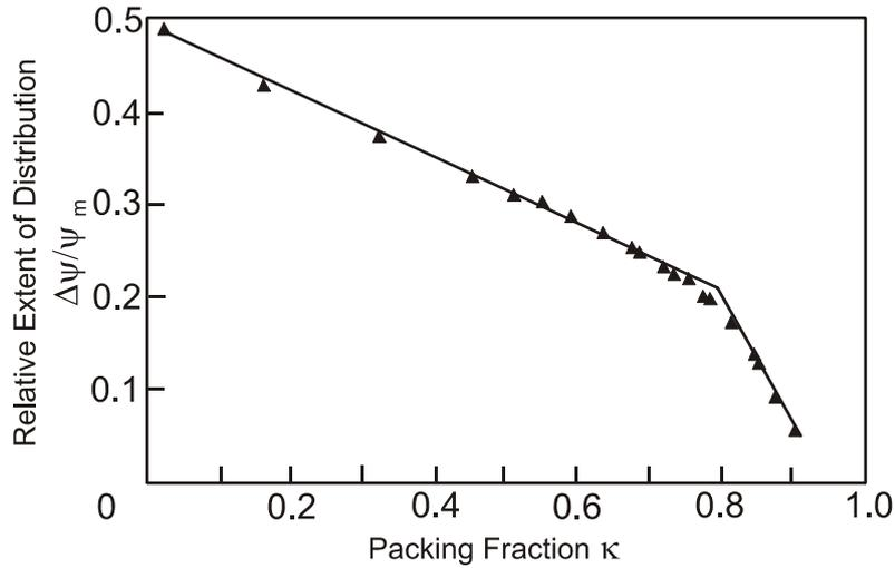
FIG. 135. Extent of contact angle distribution in dependency of packing fraction (monosized cylinders)
