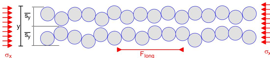
FIG. 105. Correction by overlapping adjacent chains
