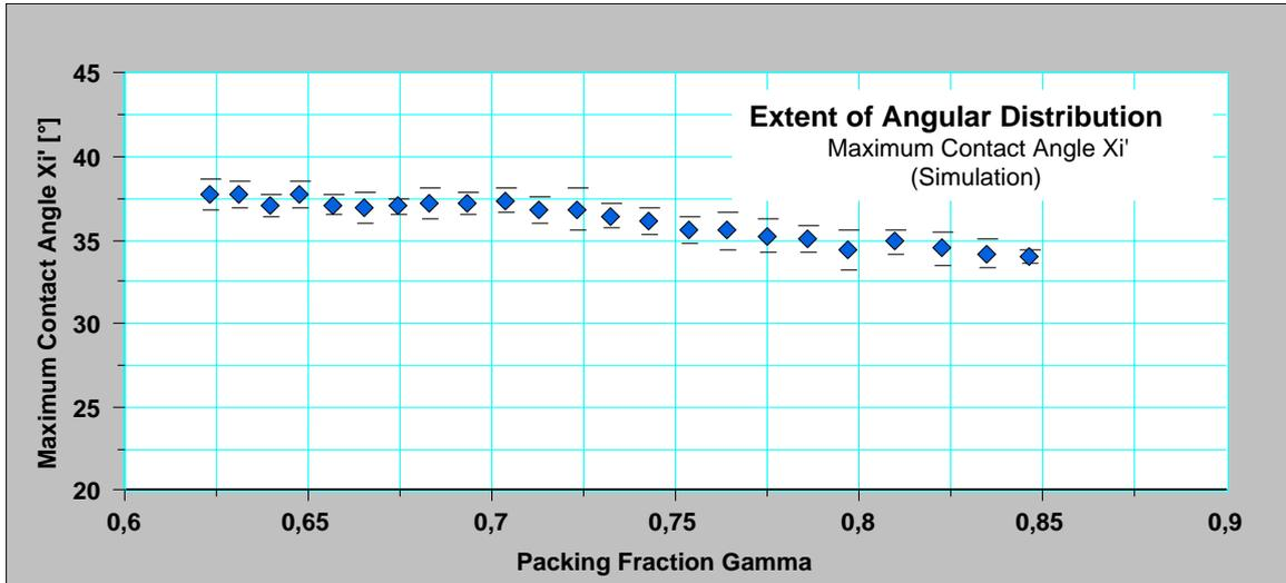
FIG. 140. Extent of the distribution of contact angles vs. Packing fraction (File: SimulationOfOrder.123)
