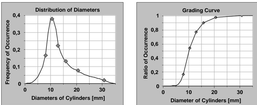
FIG. 12. 2D-model of granular material: Distribution of diameters. (File: FrequencyOfSize.123)
