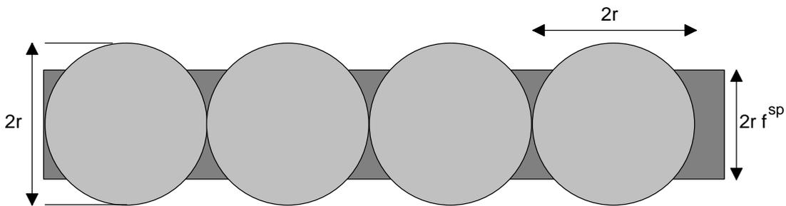
FIG. 46. Correction due to the circular shape of the grains
