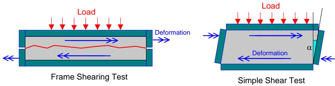
FIG. 4. Experiments enforcing a given shear joint
