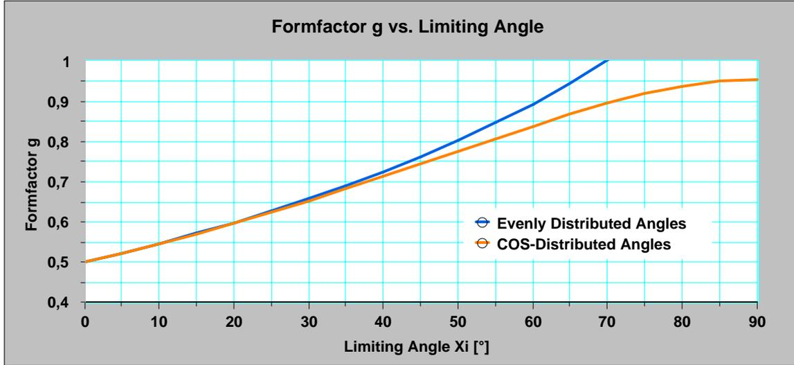
FIG. 98. Form factor  $g$  derived from the extent of a 'basic cell' (File: Formfactor, General.123)
