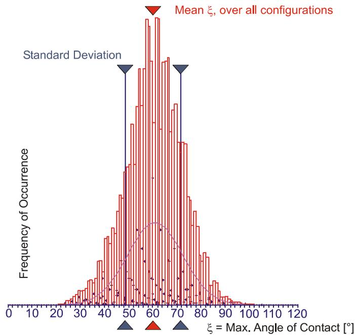
FIG. 89. Numerically obtained distribution of maximum angle of contact, based on the set of cylinders used here.
