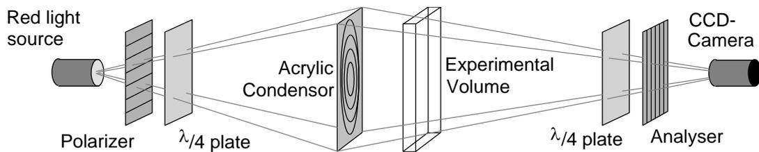
FIG. 14. Schematic view of the polariscope setup
