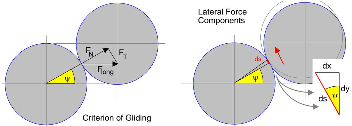
FIG. 129. Redirection of forces in preliminary model
