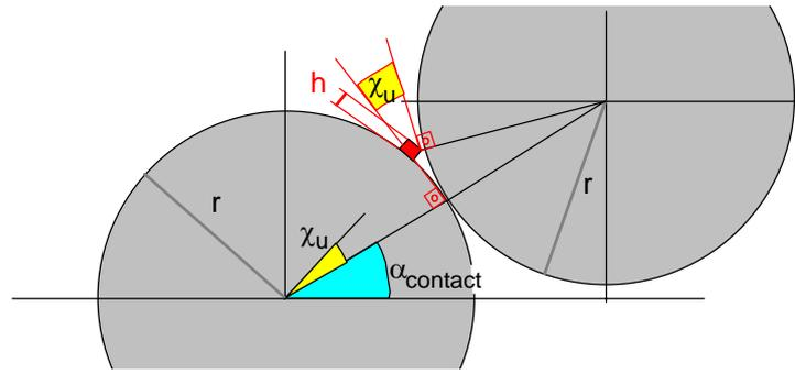
FIG. 75. Unevenness on the cylinder surface characterized by its height
