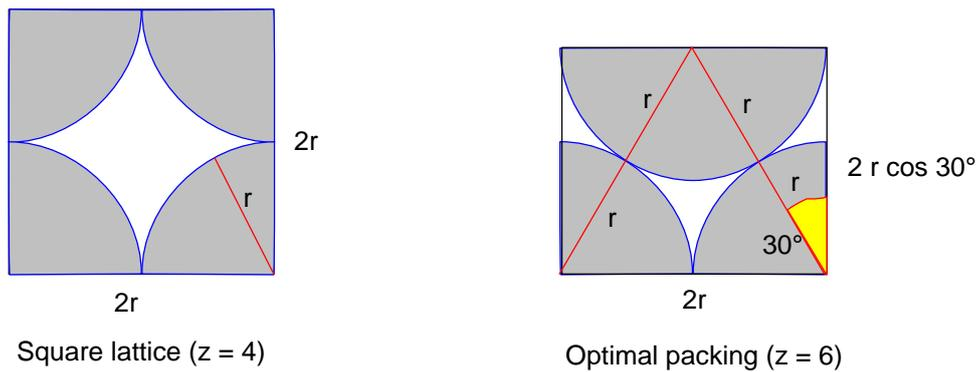
FIG. 50. Theoretical porosity values of square and optimal lattices
