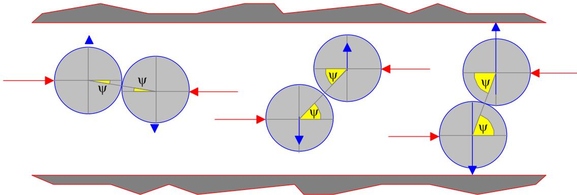
FIG. 95. Stopping probability depending on angle of contact  $\psi$
