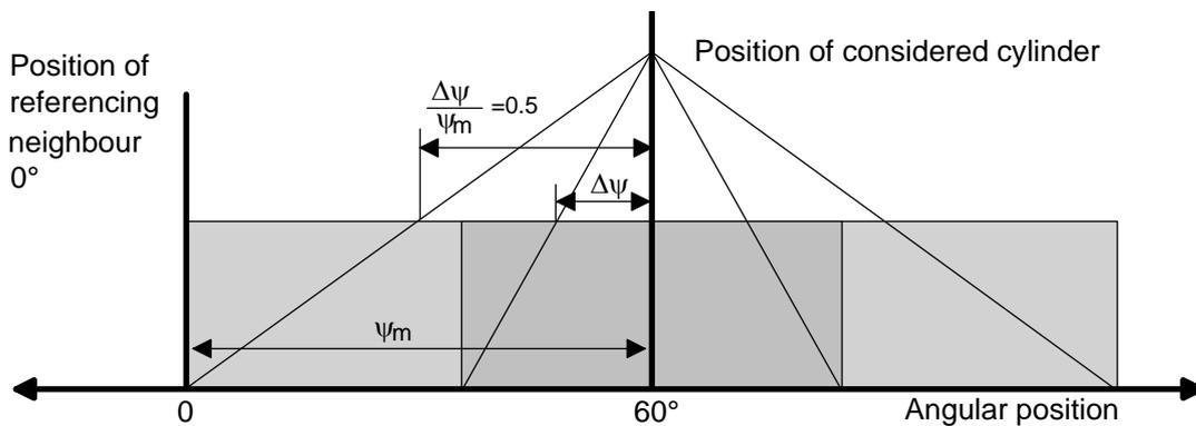
FIG. 136. Extent of contact angle distribution for infinite packing fraction (monosized cylinders)
