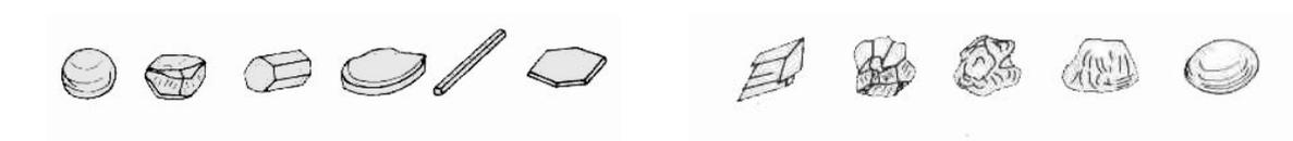
FIG. 8. Different Shapes and Roughness of Granules in Natural Soil (according to [58])
