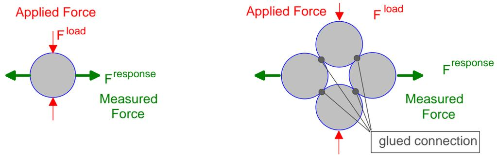
FIG. 27. Schematic view of measurement setup in order to obtain the elastic contribution
