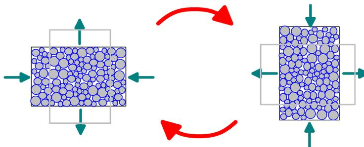
FIG. 36. Procedure to experimentally produce a minimum porosity for the granular model used here
