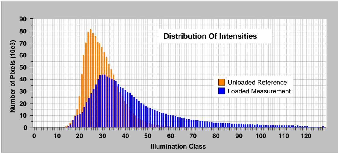
FIG. 42. Exemplarily shown distribution of light intensities  $W_{Load}(\omega)$  and  $W_0(\omega)$ (File: Demo-TCN-Distrib.123)
