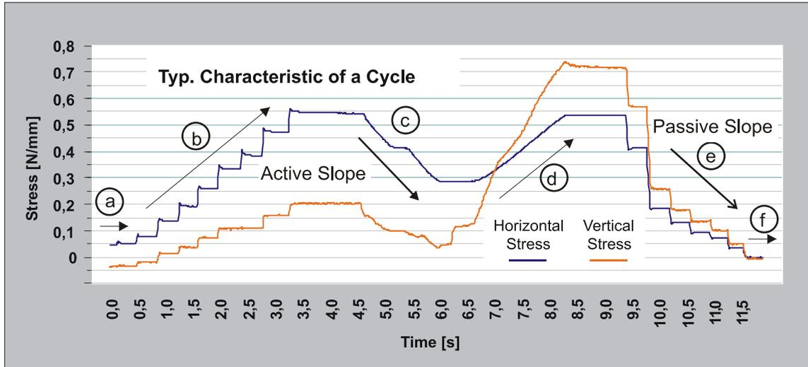
FIG. 33. Exemplary measurement I results confirming the achievement of an active state (File: PassV13 Diagram Disp.123)
