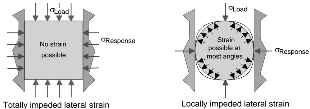
FIG. 28. Different consequences of impeded horizontal strain on rectangular and circular elements
