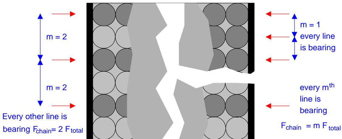
FIG. 145. Condition of equilibrium in inhomogeneous granular material
