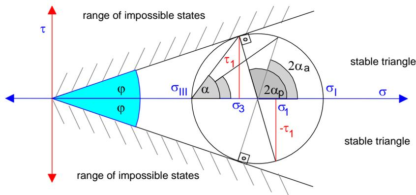
FIG. 60. The Rankine border states, shown on the Circle of Mohr-Coulomb
