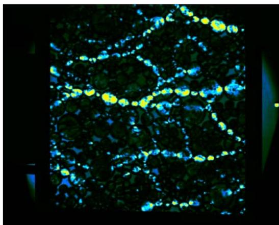
FIG. 15. Exemplary processed image, where the colour transition to yellow indicates bearing forces
