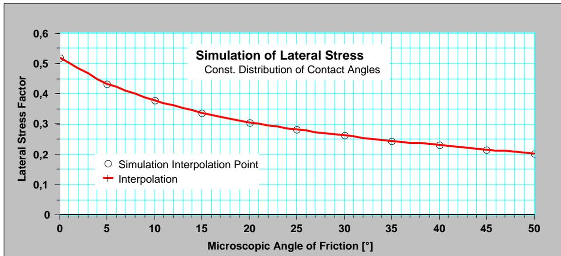
FIG. 101. Averaged lateral stress factor, using a constant distribution (File: NumSimulation.123)
