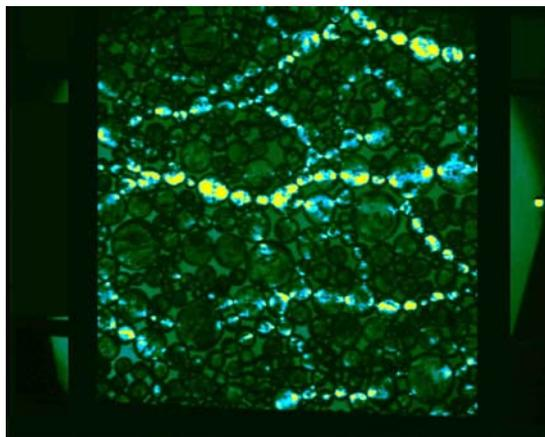
FIG. 29. Typical polariscope picture, indicating no exceeding stress at the corners
