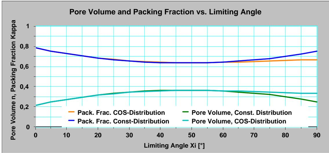
FIG. 99. Pore Volume  $n$  and packing fraction  $\gamma$  derived from the extent of a 'basic cell' (File: Formfactor, General.123)
