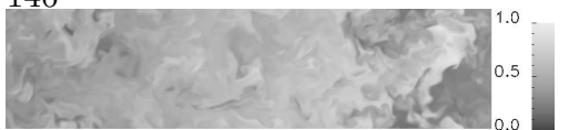
Figure 2.20: Case inert-0.7: Instantaneous mass fraction field of O_2 , x_1 - x_2 -plane in the middle of the computational domain at \tau_\omega = 697
