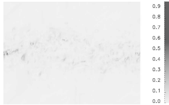
Figure 2.197: Case inert-1.1: Instantaneous pressure gradient field, x_1 - x_3 -plane through x_2 = 0.59L_2 at \tau_\omega = 1295 . Pressure gradient is normalized by \delta_{\omega,0}/\langle p \rangle_{av}
