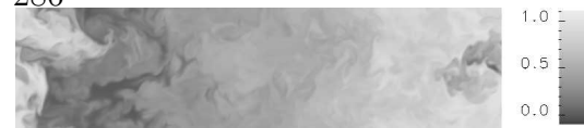
Figure 2.9: Case inert-0.15: Instantaneous mass fraction field of O_2 , x_1 - x_2 -plane in the middle of the computational domain at \tau_\omega = 533
