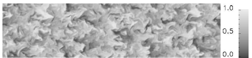
Figure 2.18: Case inert-0.7: Instantaneous mass fraction field of O_2 , x_1 - x_2 -plane in the middle of the computational domain at \tau_\omega = 146
