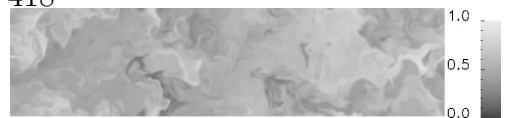
Figure 2.21: Case inert-0.7: Instantaneous mass fraction field of O_2 , x_1 - x_2 -plane in the middle of the computational domain at \tau_\omega = 980
