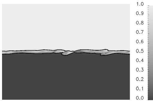
Figure 2.26: Case inert-1.1: Instantaneous mass fraction field of O_2 , x_1 - x_3 -plane in the middle of the computational domain at \tau_\omega = 162 , isolines Y_{O_2} = 0.1 and 0.9 are shown
