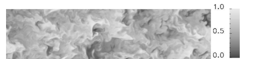
Figure 2.31: Case inert-1.1: Instantaneous mass fraction field of O_2 , x_1 - x_2 -plane in the middle of the computational domain at \tau_\omega = 381
