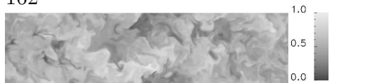
Figure 2.32: Case inert-1.1: Instantaneous mass fraction field of O_2 , x_1 - x_2 -plane in the middle of the computational domain at \tau_\omega = 735
