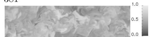
Figure 2.33: Case inert-1.1: Instantaneous mass fraction field of O_2 , x_1 - x_2 -plane in the middle of the computational domain at \tau_\omega = 1098
