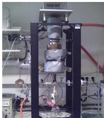
Figure B.3: Experimental set-up for adsorption isotherm measurements in Leipzig.
