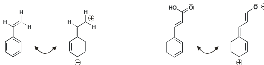
Figure 59: main resonance structures of vinylbenzene (left) and cinnamic acid (right); vinyl substituents exhibit considerable electron-donating properties which do not appropriately reflect the rather electron-withdrawing capacity of the vinyl-carboxylic acid.
