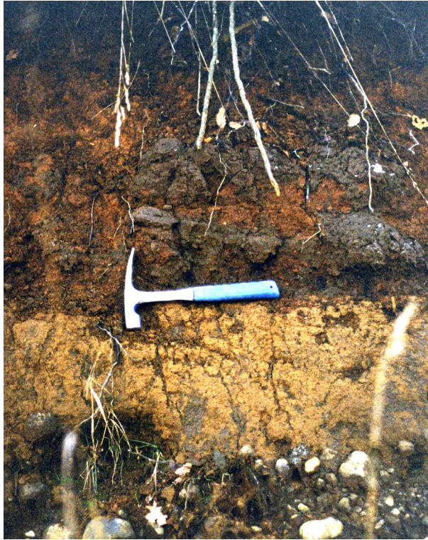
Fig. III-6: Strongly altered volcanic soils near the southern side of Lago Villarrica. Locally, they have formed clay-like soils with nearly water impenetrable blankets of weathered volcanic ashes. Location is indicated in Fig. III-3b.
