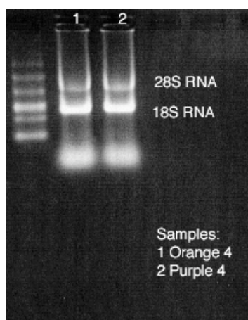
Figure 4.9: Total RNA isolated using the Trizol reagent after homogenisation with a syringe. Samples were separated in the 1.2 % agarose-formaldehyde gel. High Range RNA ladder ® was used as size standard.
