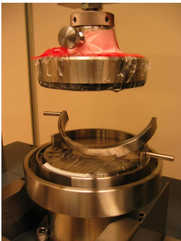
Figure 4.1: Experimental set-up showing the soft coverage of the upper plate, split rings, wax, and the milled out center piece.
