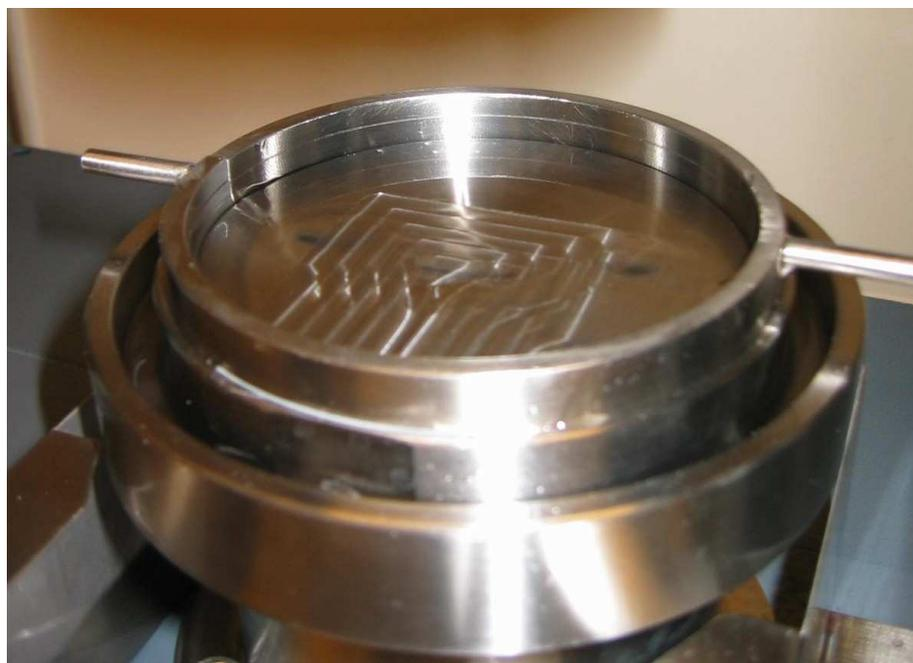
Figure 4.5: Bottom plate of the set-up with milled-out center in the shape of the sensor, depth  $100\ \mu\text{m}$ .
