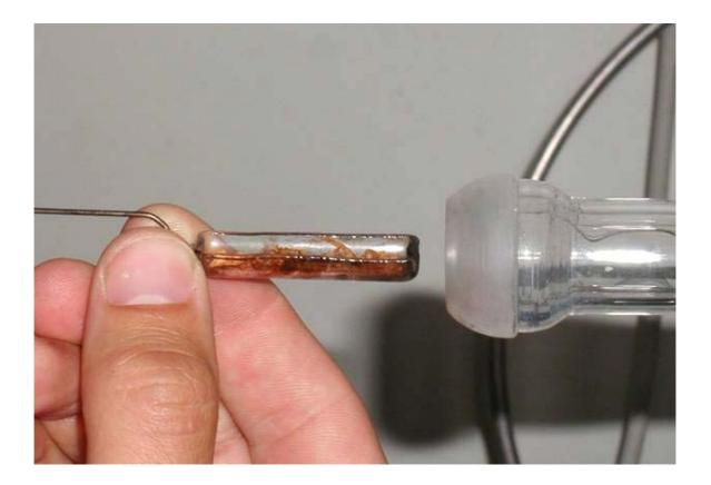
Figure 19: Photograph of the quartz boat containing a tobacco sample taken before being pushed into the quartz tube of the pyrolysis furnace
