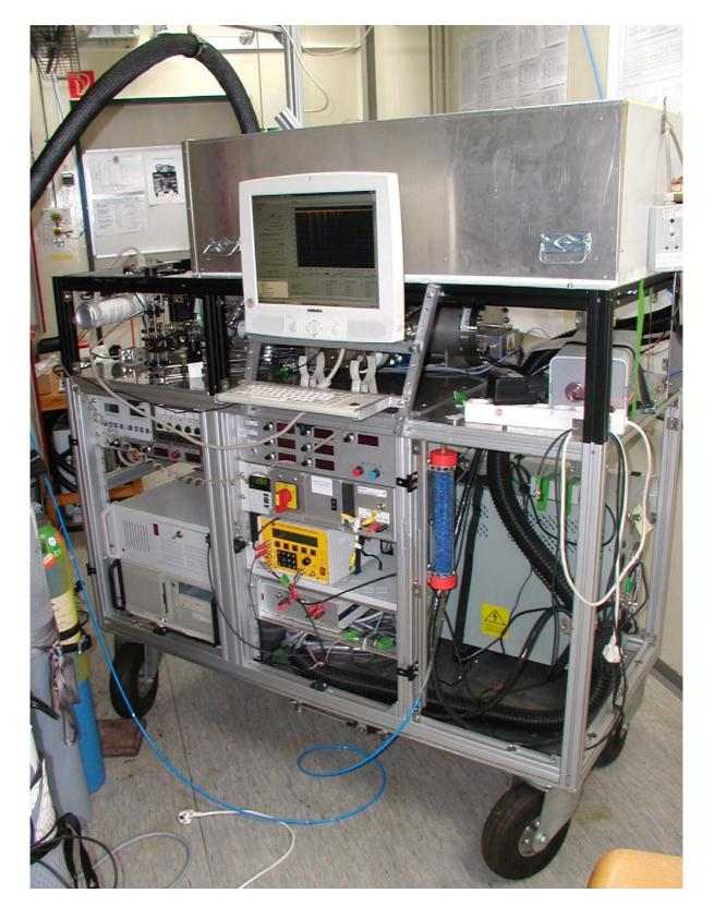
Figure 13 A: Photograph of the SPI/REMPI/EI-TOFMS instrument which was used for all the experiments in this work
