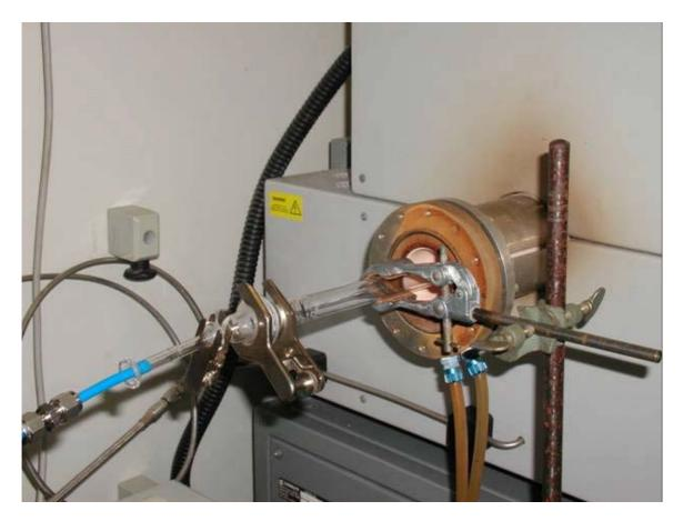
Figure 18: Inlet of the pyrolysis furnace and the quartz tube with the reaction gas line connected to the tube
