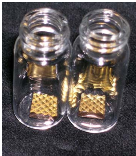
Square structure (for a square cell in chip) Pyramids larger but with small height
