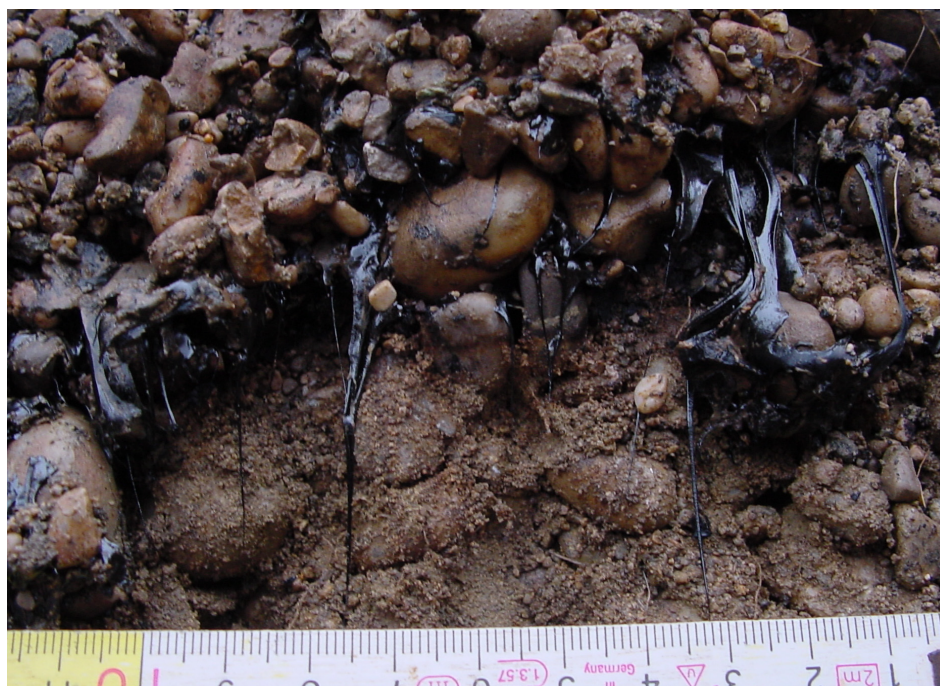
Figure 3 Coal tar at the field site. The integrity of the aged NAPL interfaces are destroyed during the excavation of the profile.
