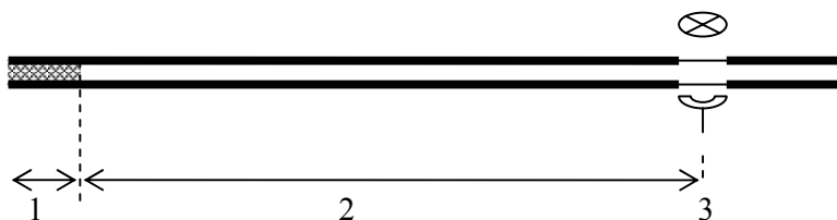
Figure 67: Scheme of the at-line pre-concentration system. Abbreviations: 1, concentrator; 2, separation and 3, detection parts.
