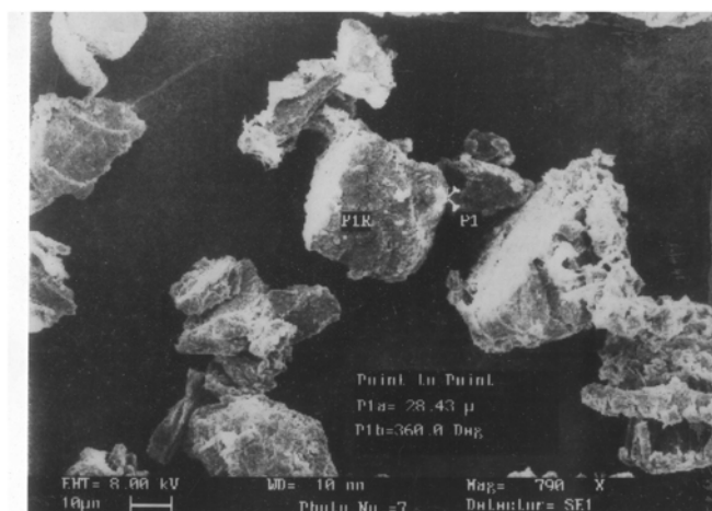
Fig. 5.28 (b): Scanning electron microscope (SEM) photograph of cryo-ground turmeric particles
