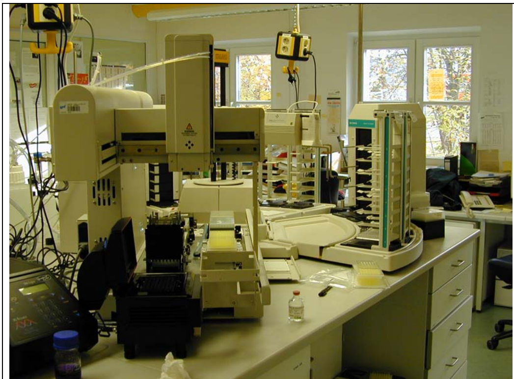
Figure 6.1.2: Biomek 2000 pipetting robot. Producing DNA probes for microarray production has to be done in high-throughput format. Programming new protocols for this machine is time consuming but worthwhile for large sample batches (like the 70.000 PCR reactions for the 21k mouse array).
