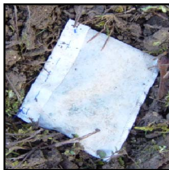
Figure 4. Litter bag of mesh size 40 \mu\text{m} (10 x 10 cm) filled with dried litter and closed by stitching before incubating in soil sites for degradation experiments.
