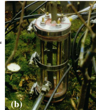
Figure 2.8a. Sketch of the open gas exchange system used to measure stem respiration. SG and RG represent sample gas and reference gas, respectively. Figure 2,8b shows a respiration-chamber attached to the stem of a beech individual.
