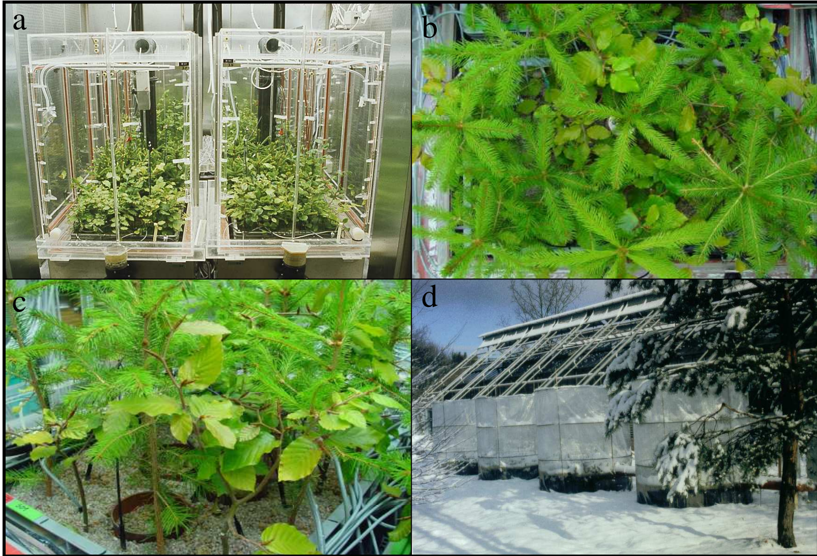
Figure 2.2. Plant containers in sub-chambers of one phytotron (a), container with mixed culture (b, c), and open-top-chambers of GSF-Research Center.
