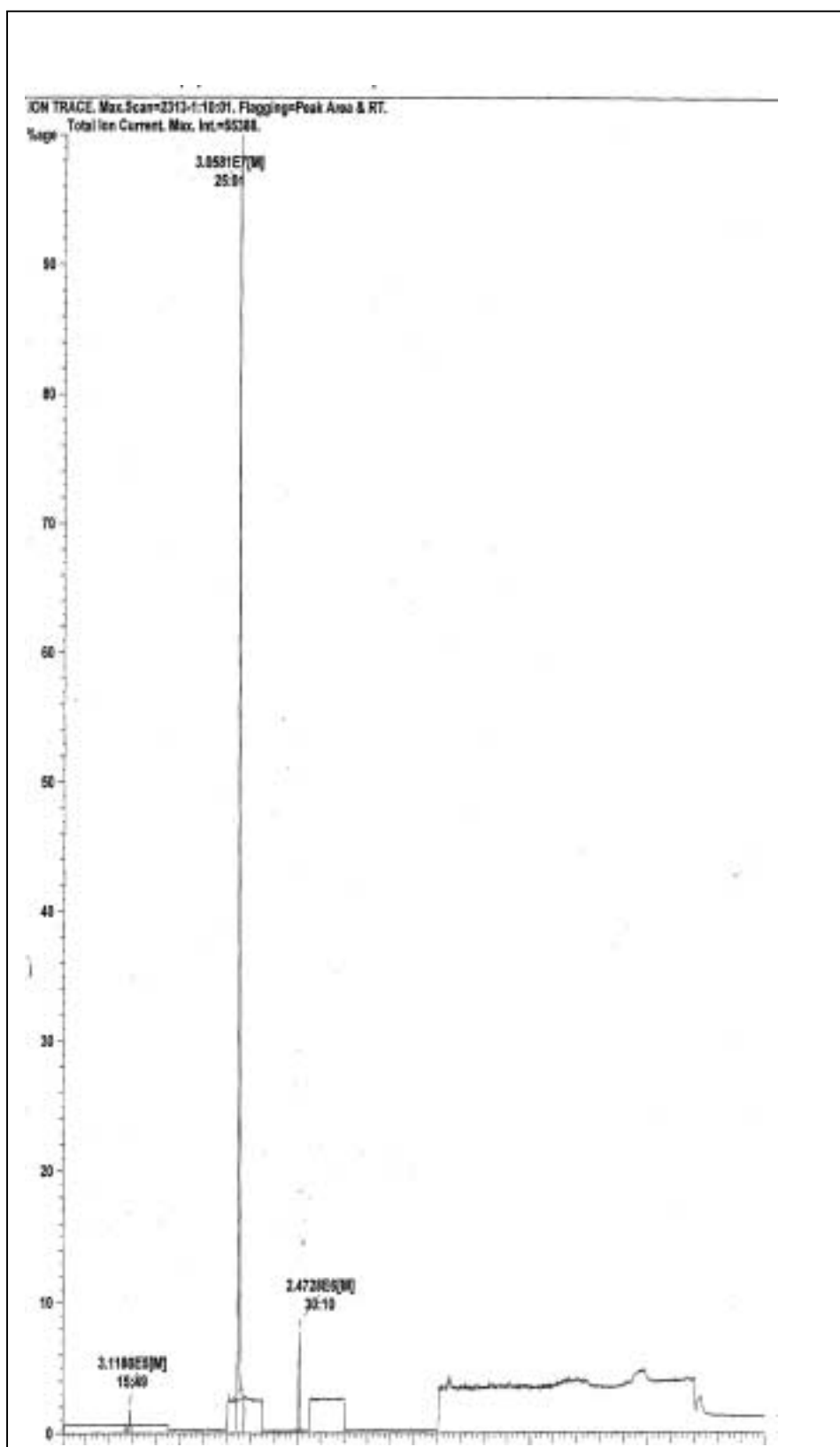
Figure 19a. Silica gel fraction 1: Total Ion Current: Total Ion current showing Lindane (Rt: 15:49), Chlorpyrifos ethyl (Rt: 25:01) and \alpha -Endosulfane (Rt: 30:10) Flagging = Peak Area & Rt
