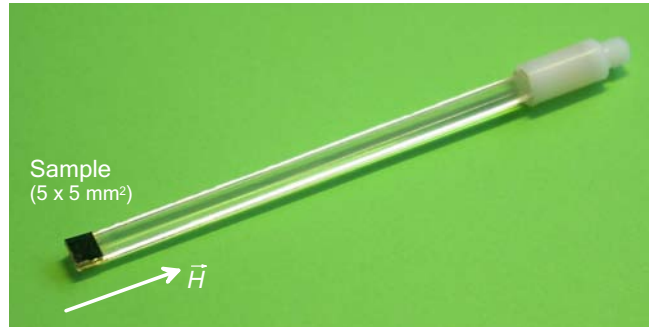
Figure 3.4: Sample holder for ACMS option of PPMS. The sample is mounted on one end of a quartz stick with a flat face. The quartz stick is fixed in an intermediate piece of polyacetal (Delrin), which allows attaching the ensemble to the standard transportation rod. Samples are glued on the sample holder using GE varnish.
