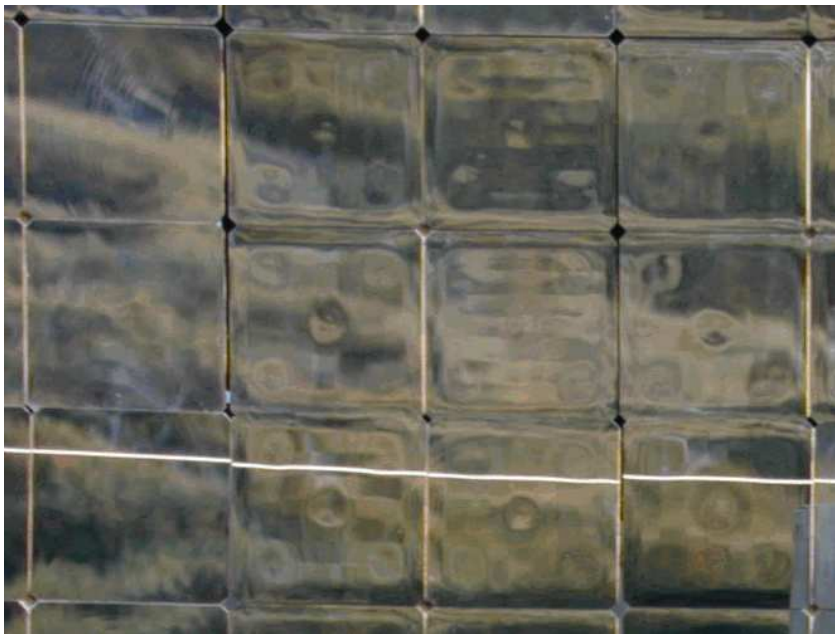
Figure 4.28: The mirror elements seen from the camera access tower, i.e. around the focal distance. The position is optimal to visualize the tiny imperfections of the surface of the mirrors. The ones on the right are M mirrors; it is possible to recognize the channel for the heating and the small central depression.
