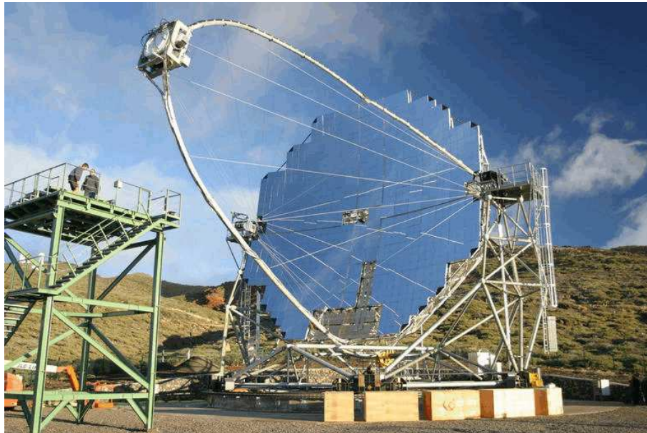
Figure 4.1: The MAGIC telescope in October 2003 (about 5% of the mirror elements is still missing).
