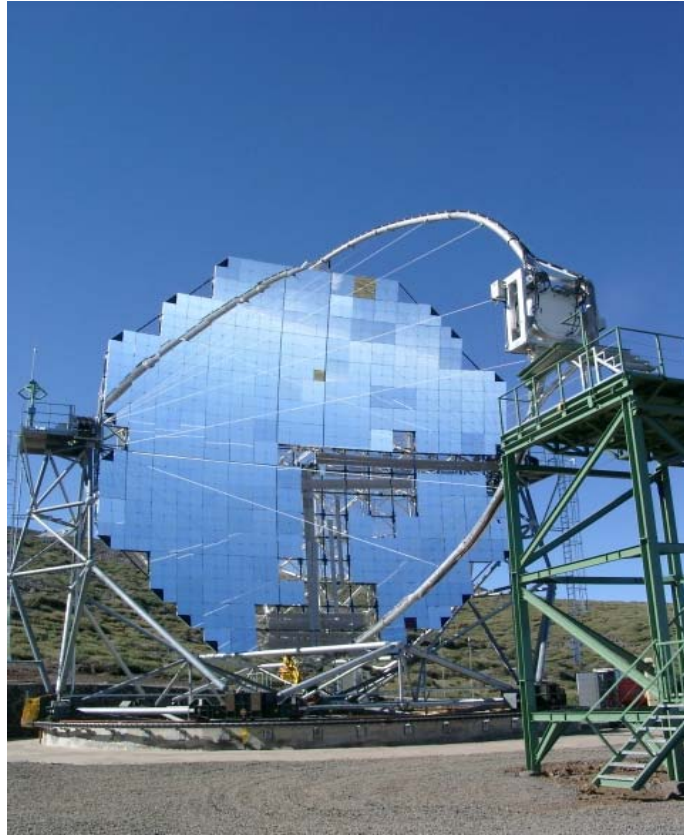
Figure 2: The MAGIC atmospheric Cherenkov telescope, for the study of very high energy \gamma rays from astrophysical sources. The CT1 telescope is the experimental precursor of MAGIC. MAGIC is the today largest atmospheric Cherenkov telescope, and has the lowest energy threshold (10-30 GeV). (Courtesy of MAGIC gallery Uni.Wuerzburg, http://www.astro.uni-wuerzburg.de/magic/gallery )
