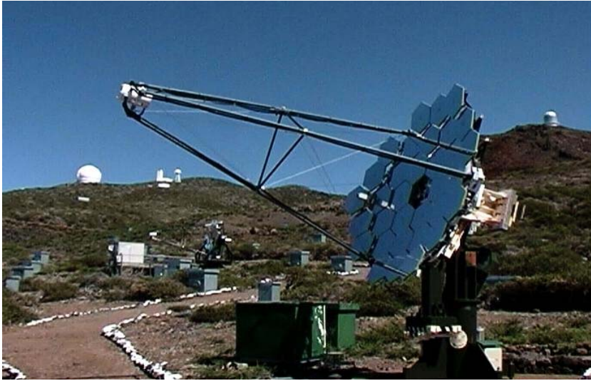
Figure 2.6: The HEGRA CT1 stand alone IACT. The CT1 is located in La Palma, Canary Islands ( 28.75^{\circ} N, 17.9^{\circ} W, 2225m. a.s.l.), at the ORM (Observatorio Del Roque De Los Muchachos). Some other telescopes of the ORM are also visible in the picture. The ORM is one of the two observatories of the IAC (Instituto de Astrofísica Canarias).
