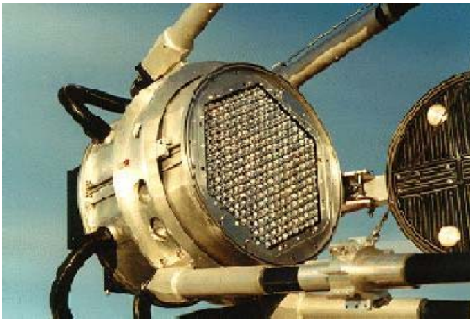
Figure 2.7: The CT1 camera. It contains 127 photo-multipliers EMI 9083A of 21 mm of diameter, with photocathode quantum efficiency of 26% at 375 nm. Each photo-multiplier covers an angular region, of hexagonal shape, with an effective diameter of 0.244^{\circ} .
