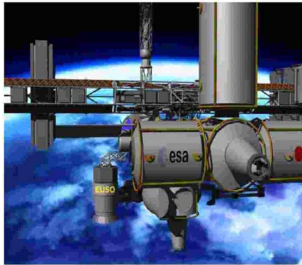
Figure 3: The future EUSO detector, for the study of the UHE cosmic rays, on board of the ISS (simulation).
