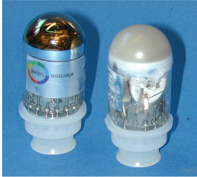
Figure 4.4: Photograph of a plain ET9116A PMT (left) and a specially coated ET9116A PMT (right). See text for further details.
