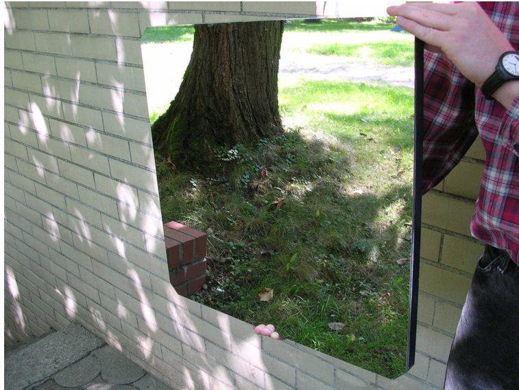
Figure 3.5: Photograph of one of the 964 mirror elements of the mirror dish of MAGIC.
