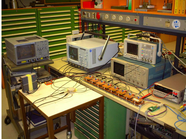
Figure D.3: Photograph of the experimental setup that was used to evaluate the performance of non-connectorized VCSELs.
