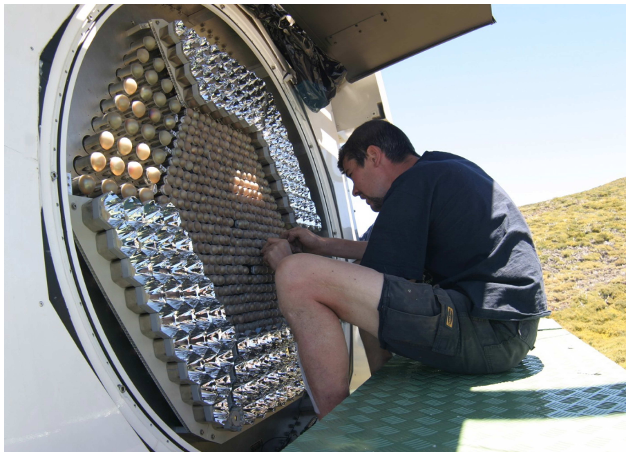
Figure 4.19: Photograph of the camera of the MAGIC Telescope during the coated PMT installation.
