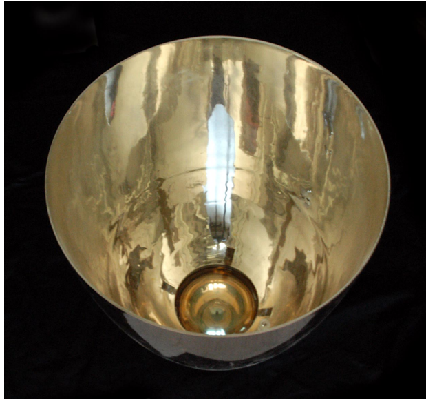
Figure 3.3: A CTF light guide. The mounted photomultiplier can be seen in the opening in the back. The front aperture has a diameter of 50.6 cm.
