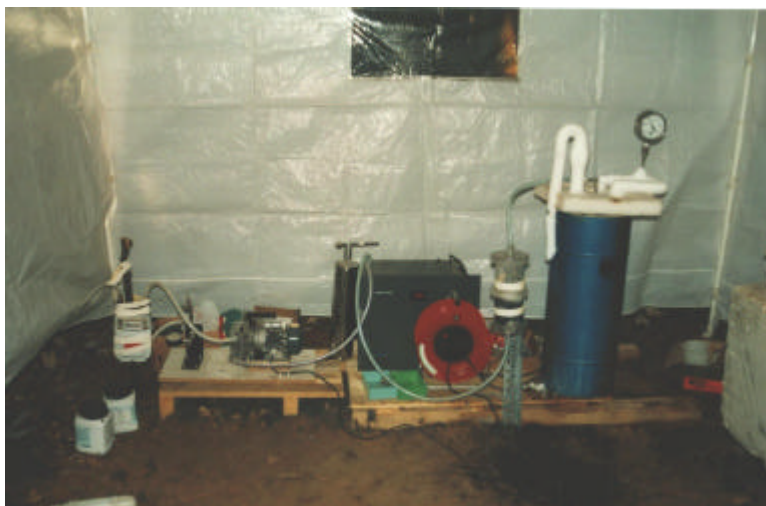
Figure 31 Experimental setup for the collection of \text{CH}_3\text{Cl} from the air in Kranzberger Forst: (left to right) gas meter, pump, pre-cooler, NaOH container, main cooler
