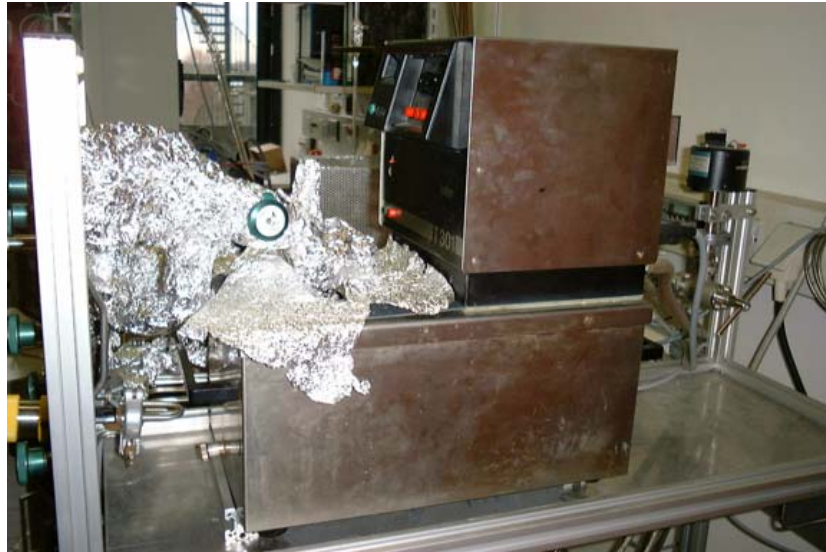
Fig. 6.4: Thermostat used to regulate the temperature of the precursor. The precursor bottle was located inside the tank with pure distilled water.
