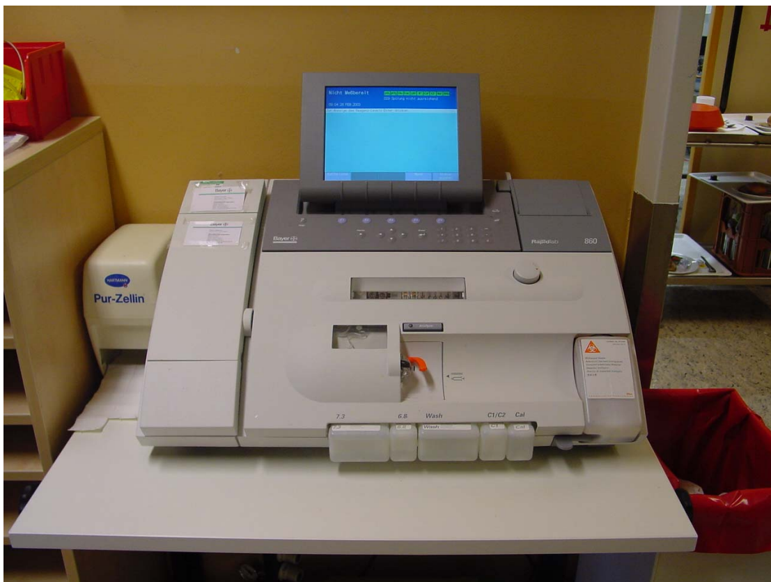
Figure 3. Arterial blood gas analyser (Bayer Rapidlab 860) was used to measure the arterial blood sampling (arterial blood gas, electrolyte, as well as hematocrit and hemoglobin).
