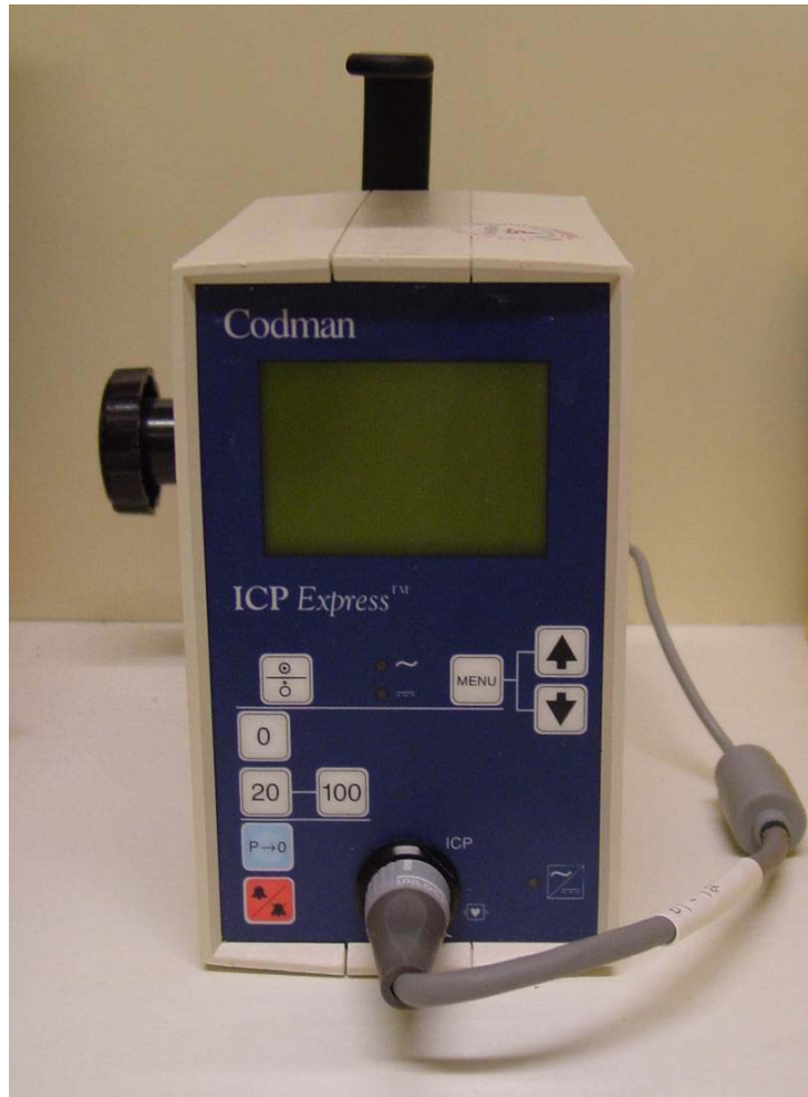
Figure 2. Intracranial pressure monitoring system (Codman ICP Express) was continuously used for ICP measuring during the time of study.
