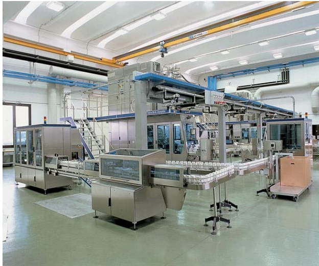
Figure H.2 TetraPak packaging line
