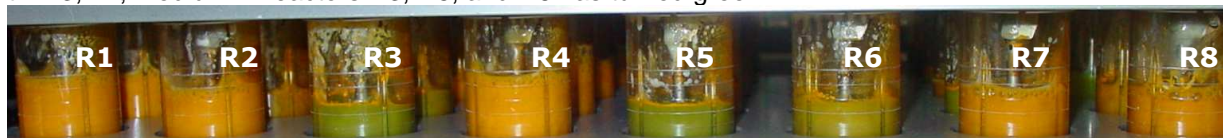
Figure 4-41: Photographs of the first column of reactors (R1-R8) with volumetric scores during a 48-fold parallel B2 cultivation at different indicated process times.
