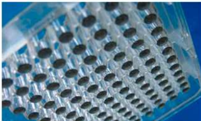
Figure 7-4: Bottom of a HydroPlate® HP96L (PreSens, Regensburg) for parallel pH measurement in 96 wells with optical shielding.
