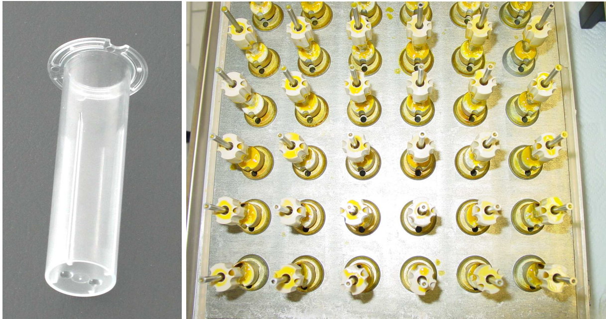
Figure 7-2: Left: Injection-molded polystyrene (PS) milliliter bioreactor with four baffles and optical lenses at the bottom intended for internally immobilized fluorescence spots. Right: Cover lid of the reaction block with 48 gas-inducing impellers on hollow axes (photographed upside down after the completion of a 48-fold B2 process).
