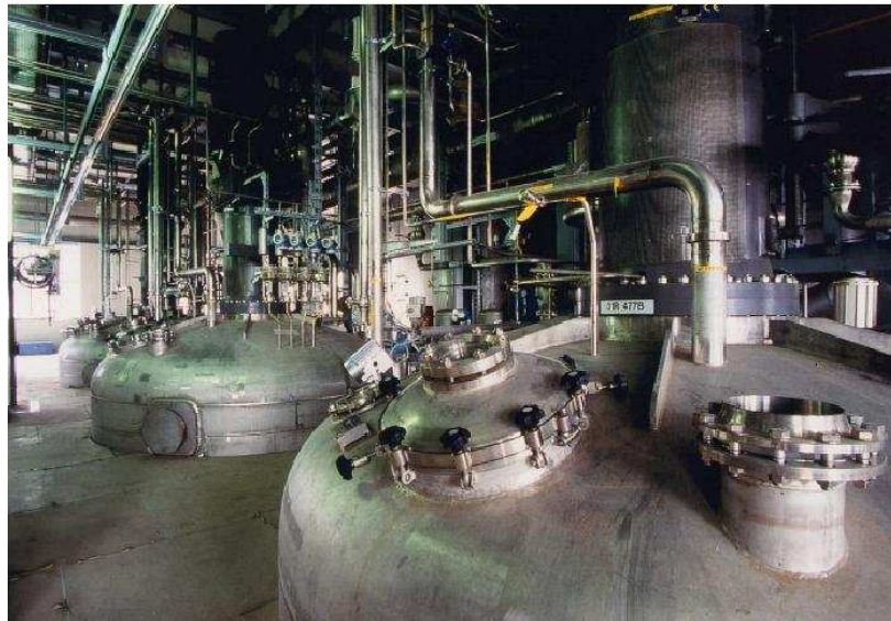
Figure 3-8: Production vessels for the biotechnological production of vitamin B2 (riboflavin) with recombinant Bacillus subtilis at DSM Nutritional Products, Switzerland.
