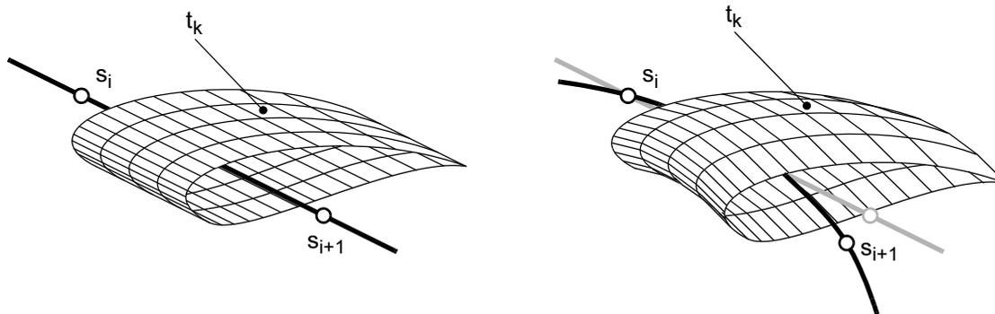
**Figure 6.3** Illustration of Mapping of Modal Deformation onto a Detailed Aerodynamic Grid With Source Points  $s_i$  and Surface Element Reference Points as Target Points  $t_k$
