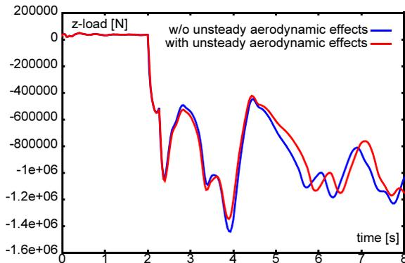
**Figure 7.13** Scenario A: Difference Between Simulation With and Without Unsteady Aerodynamic Effects (Aerodynamic Excitation / Damping)
