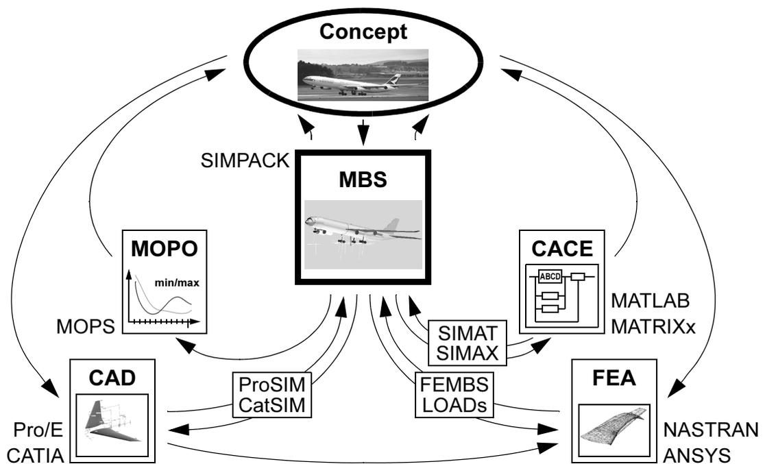
**Figure 2.2** Multibody Simulation in a Concurrent Engineering Environment
