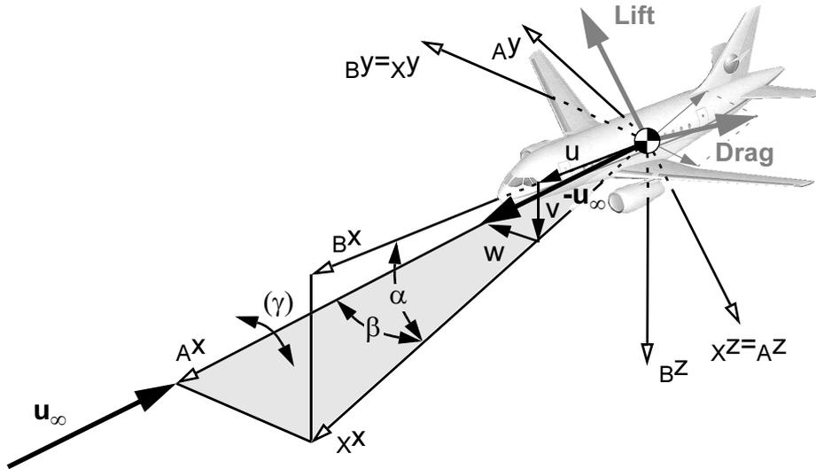
**Figure 5.4** Flight Attitude Measurements for the Vector of Rigid Body States
