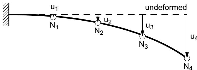
Figure 5.11 1<sup>st</sup> Bending Mode of a Cantilever Beam
