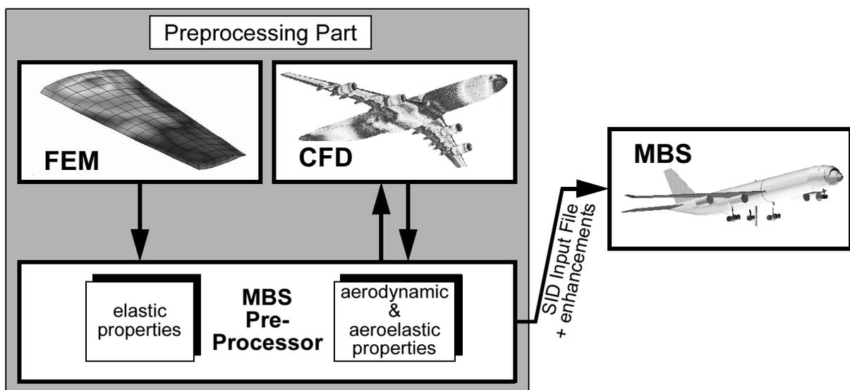
**Figure 3.2** Flow Scheme of Aeroelastic Preprocessing
