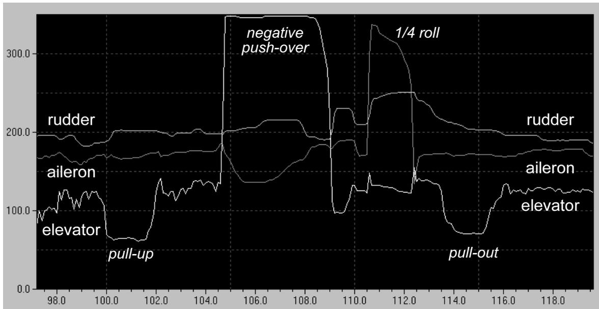
Figure 7.2 Control Inputs for an Aerobatic Manoeuvre (Humpty-Bump with  $1/4$ -Vertical Roll)
