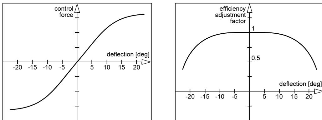
Figure 5.5 Example of Control Efficiency Function and Corresponding Efficiency Factor
