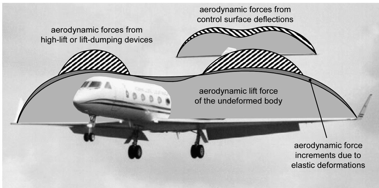
**Figure 5.1** Superposition of Aerodynamic Effects
