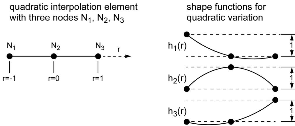
**Figure 6.5** Unidirectional Interpolation Element (Origin of Local Coordinate System at Centre Node) for Quadratic Variation
