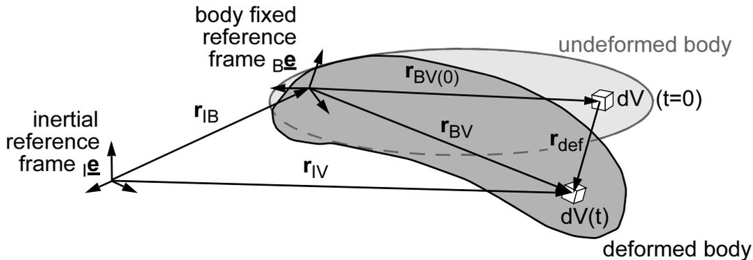
Figure 4.1 Deformation of a Deformable Body
