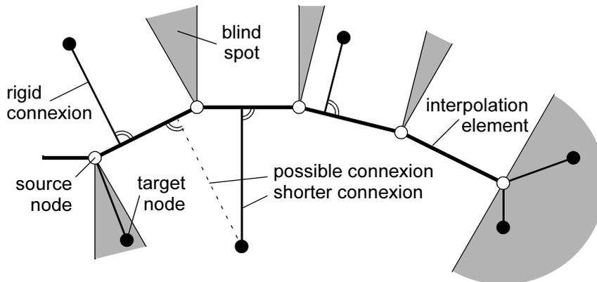
**Figure 6.7** Example of Coupling With Perpendicular Rigid Connexions
