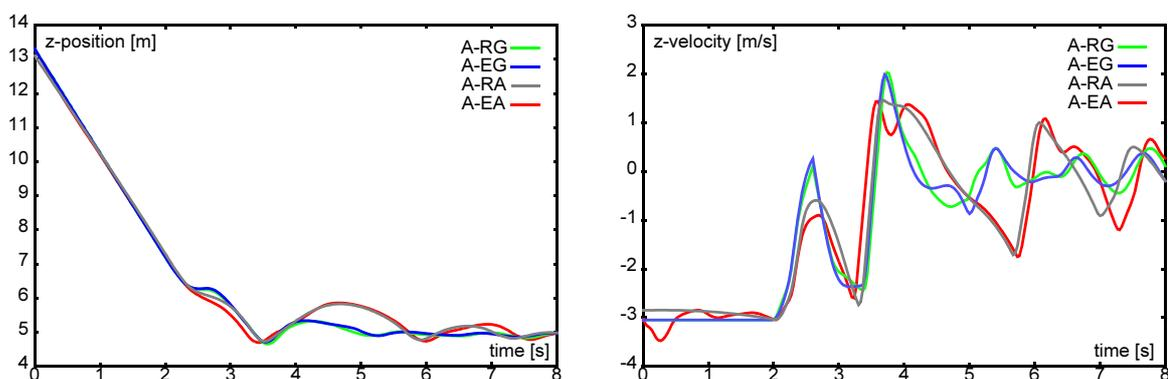
**Figure 7.5** Scenario A: Vertical Position (left) and Descent Velocity (right) of Aircraft Reference Frame Over Time
