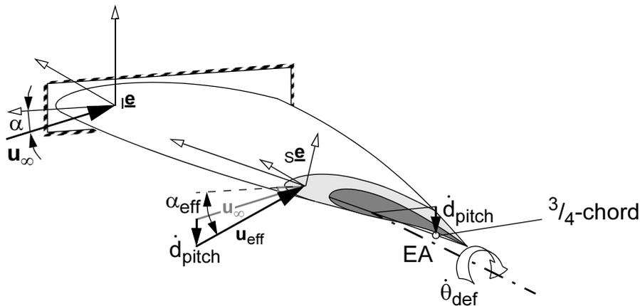
**Figure 5.9** Kinematic Velocities at a Wing Section Under Consideration of Dynamic Wing Torsion
