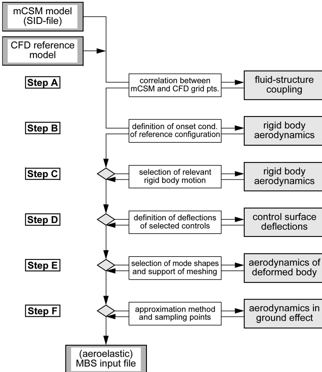
Figure 6.1 Overview of Workflow of Aeroelastic Preprocessing Using Modal Aerodynamics
