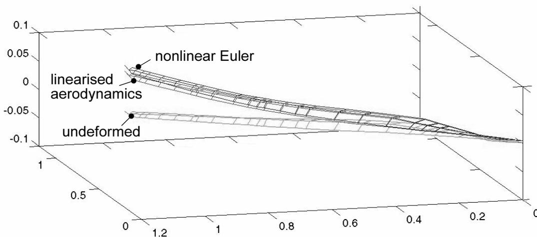
**Figure 5.2** AMP Wing - Unloaded and with Linearised and Nonlinear Aerodynamics
