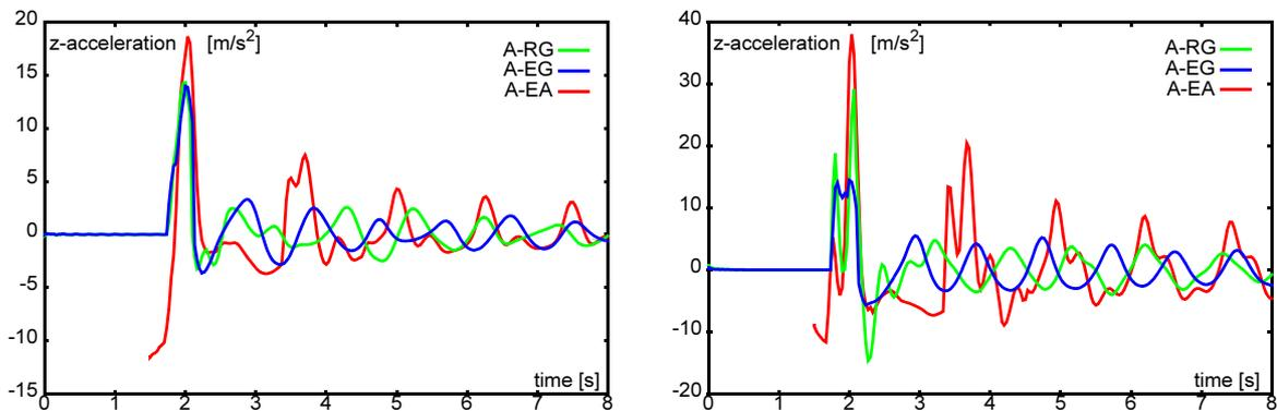
**Figure 7.7** Scenario B: Vertical Acceleration of Aircraft Reference Point (left) and of Cockpit (right) Over Time
