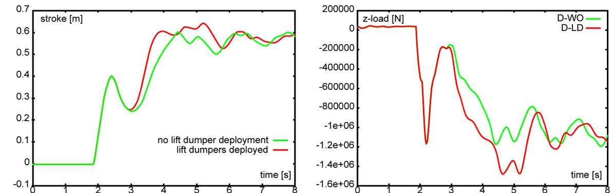
**Figure 7.12** Scenario D: Stroke of Left Main Landing Gear Oleo (left) and Vertical Load on Left Main Landing Gear Mainfitting (right) Over Time
