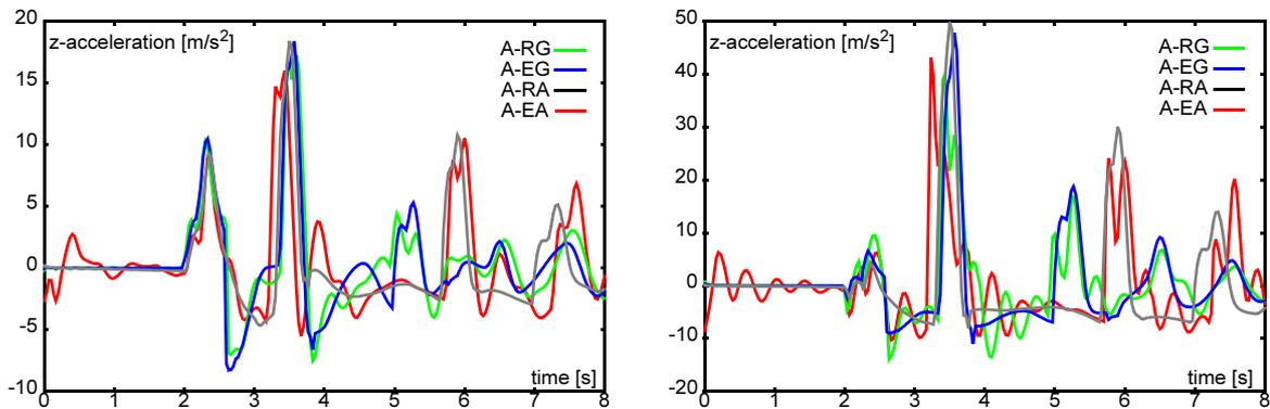
**Figure 7.6** Scenario A: Vertical Acceleration of Aircraft Reference Point (left) and of Cockpit (right) Over Time
