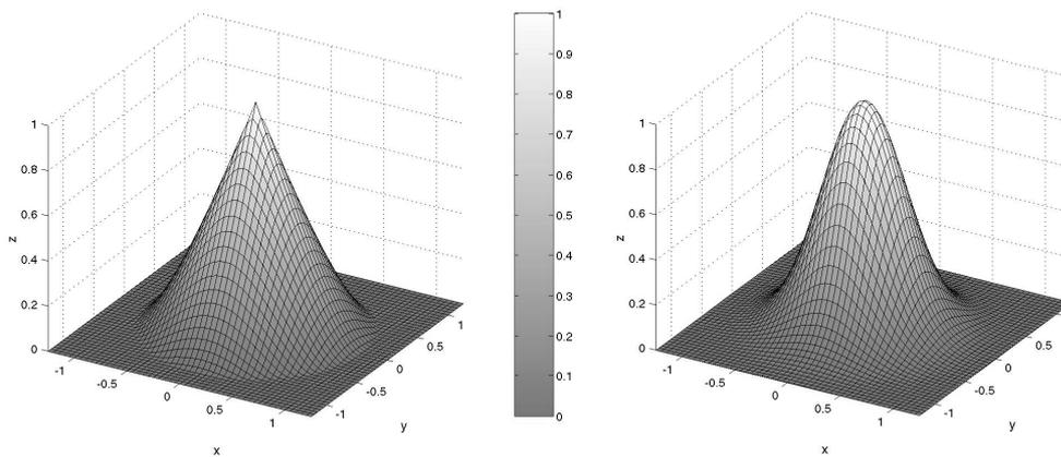
**Figure 6.6** Normalised Euclid’s Hat (left) and Gaussian Function (right) as Examples for Compactly Supported Radial Functions
