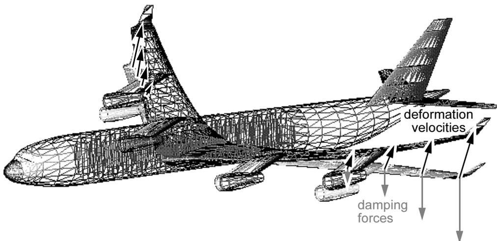
**Figure 5.10** Analysis of Aerodynamic Damping/Excitation by Characteristic Base Function (1<sup>st</sup> Wing Bending Mode)
