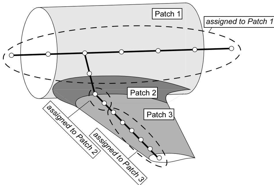
**Figure 6.8** Pre-assignment Between Interpolation Points Using Patches of the CFD Model
