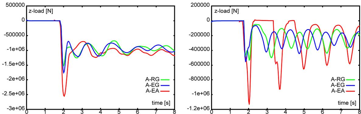
**Figure 7.10** Scenario B: Vertical Load on Left Main Landing Gear Mainfitting (left) and Nose Landing Gear Mainfitting (right) Over Time
