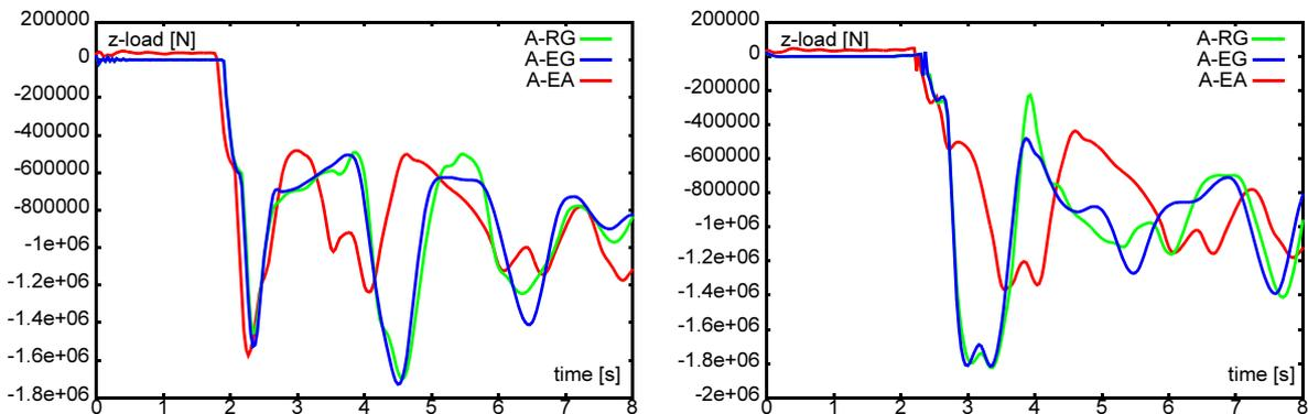
**Figure 7.11** Scenario C: Vertical Load on Right (left) and Left (right) Main Landing Gear Mainfitting Over Time
