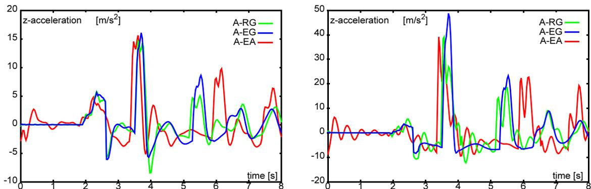
**Figure 7.8** Scenario C: Vertical Acceleration of Aircraft Reference Point (left) and of Cockpit (right) Over Time
