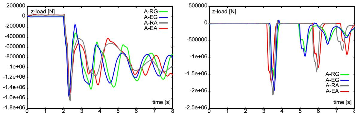
**Figure 7.9** Scenario A: Vertical Load on Left Main Landing Gear Mainfitting (left) and Nose Landing Gear Mainfitting (right) Over Time
