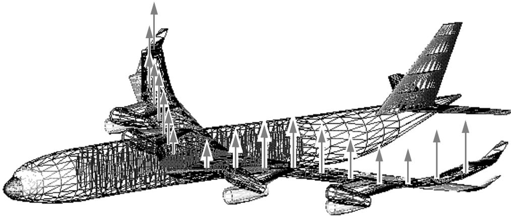
**Figure 5.7** Aerodynamic Analysis of Flexible Body Deformed by Characteristic Base Function (1<sup>st</sup> Wing Torsion Mode - deformation is overscaled)
