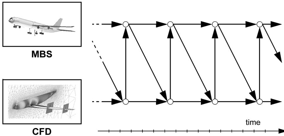
**Figure 2.7** Inter-Process Communication (IPC) Between MBS and CFD
