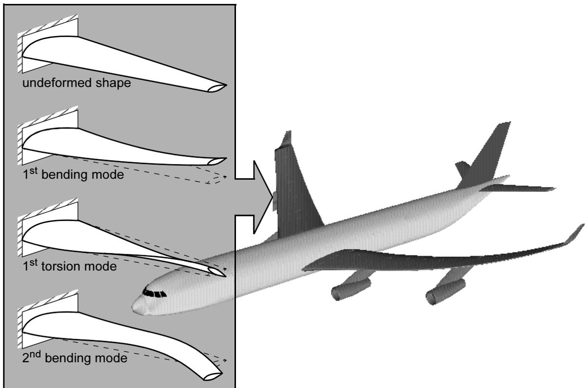
**Figure 5.3** Superposition of Basic Deformation Modes of a Deformable Body
