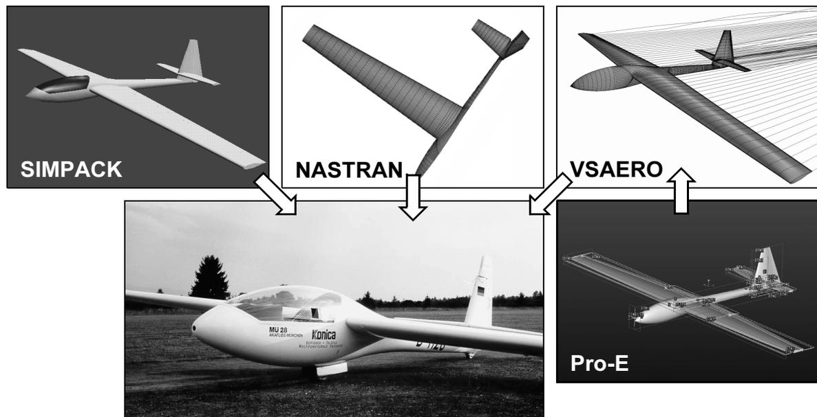
**Figure 7.1** Set-Up of Reference Model 1 Basing on Data of Mü 28 (Akaflieg München)
