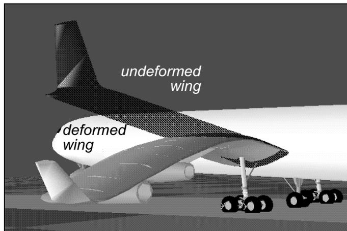
**Figure 3.1** Deflection of an A340-300 Wing at a Hard Touch-Down (10 fps-landing at MLW)
