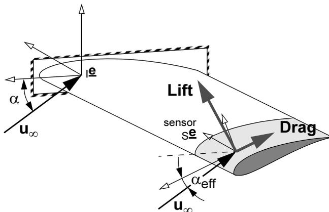
**Figure 5.6** Lift and Drag of a Wing Section Under Consideration of Wing Torsion
