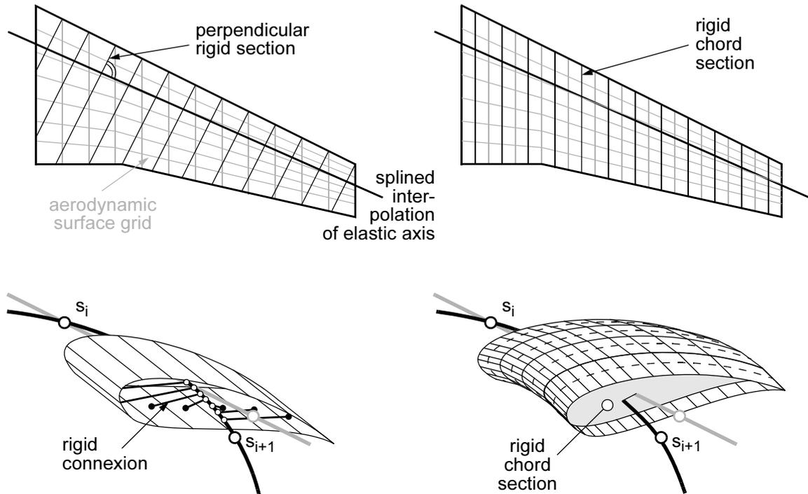
Figure 6.4 Approach of Rigid Connexions (left) and Approach of Rigid Chord Sections (right)
