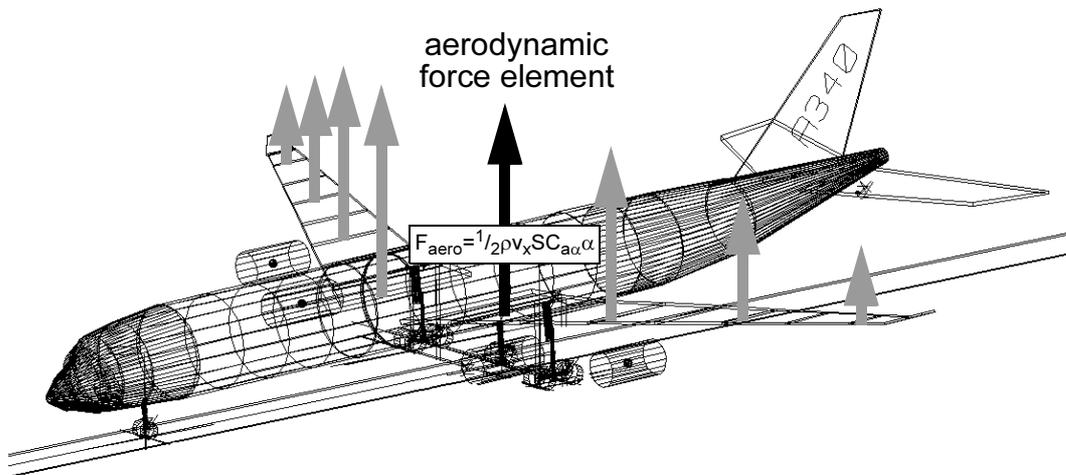
**Figure 2.6** *Distributed Aerodynamic MBS Force Elements on MBS Model*
