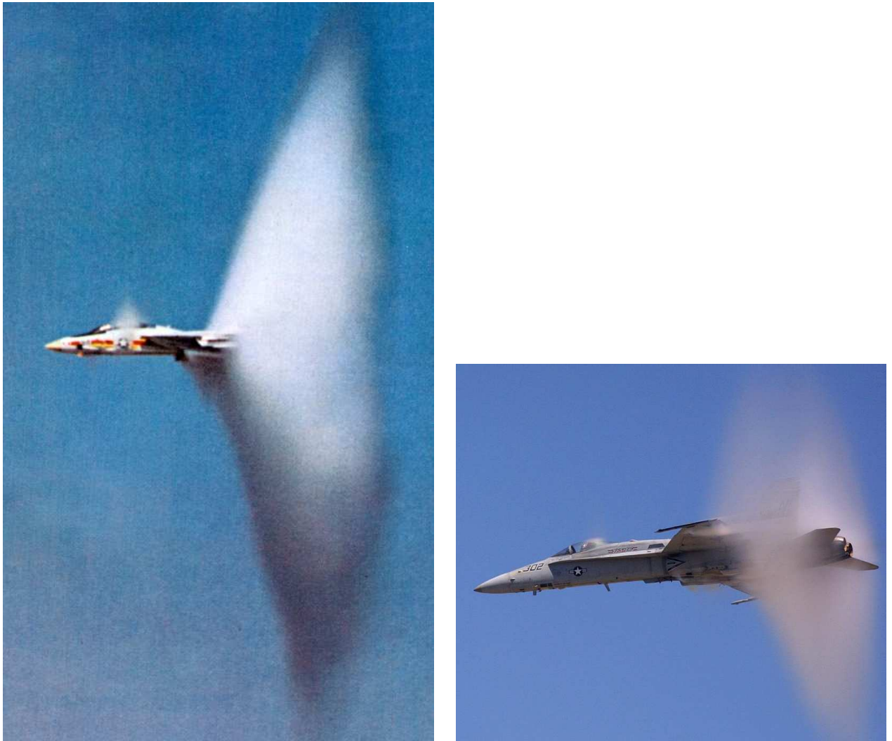
Figure 1.2.: Left: Condensation on a F-14 Tomcat during level flight at M_\infty = 0.9 [13] Right: Condensation on a F-18 Hornet, photo by Nich Chinn, at Moffet Field airshow, 2001 [19]
