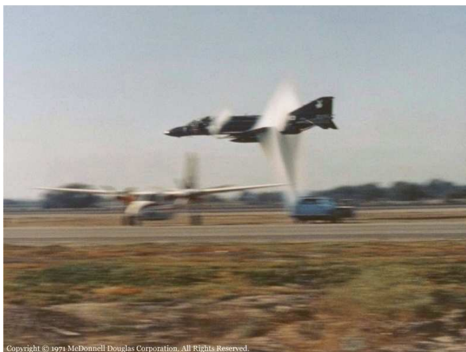
Figure 1.7.: Condensation on a F-4J Phantom II. The following paragraph is text that was written on top of the photo: This one of a kind photo was shot by Mr. Harry Gann, of McDonnell Douglas, at the Point Mugu Naval Air Station on 23 October 1971. The aircraft, a McDonnell Douglas F-4J Phantom II "Black Bunny" from Navy flight test squadron VX-4, was captured on film while flying at near supersonic velocity. However, the local velocity on parts of the aircraft were supersonic, causing the two distinctive, diamond-shaped shock wave cones around the leading and trailing edges of the aircraft. A photograph like this is rare, it required split-second timing and a large amount of luck. "At the time, I was using a motorized Nikon F-2 camera, with a 300mm lens," states Mr. Gann, "I shot about four frames. The film was Ektachrome 400. As I remember, I was standing about 70 yards from the taxiway during the pass." [90]
