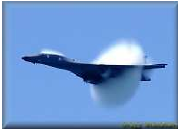
Figure 1.3.: Condensation on a B1-B Lancer, photo taken by Gregg Stansberry at Pensocola Beach, Florida, July 12, 2002 [90]
