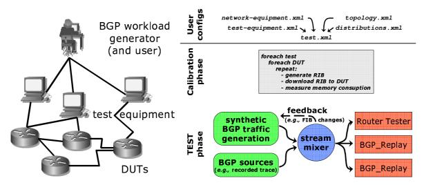
Figure 7.1: Test-bed for router testing. Figure 7.2: Overview of synthetic BGP traffic algorithm.
