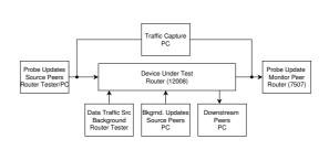
Figure 6.4: Test-bed setup for router testing.
