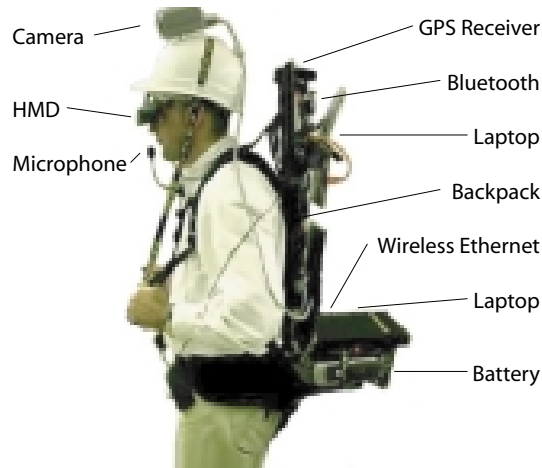
Figure 5.10: A side view of our prototype wearable computer built with DWARF.
