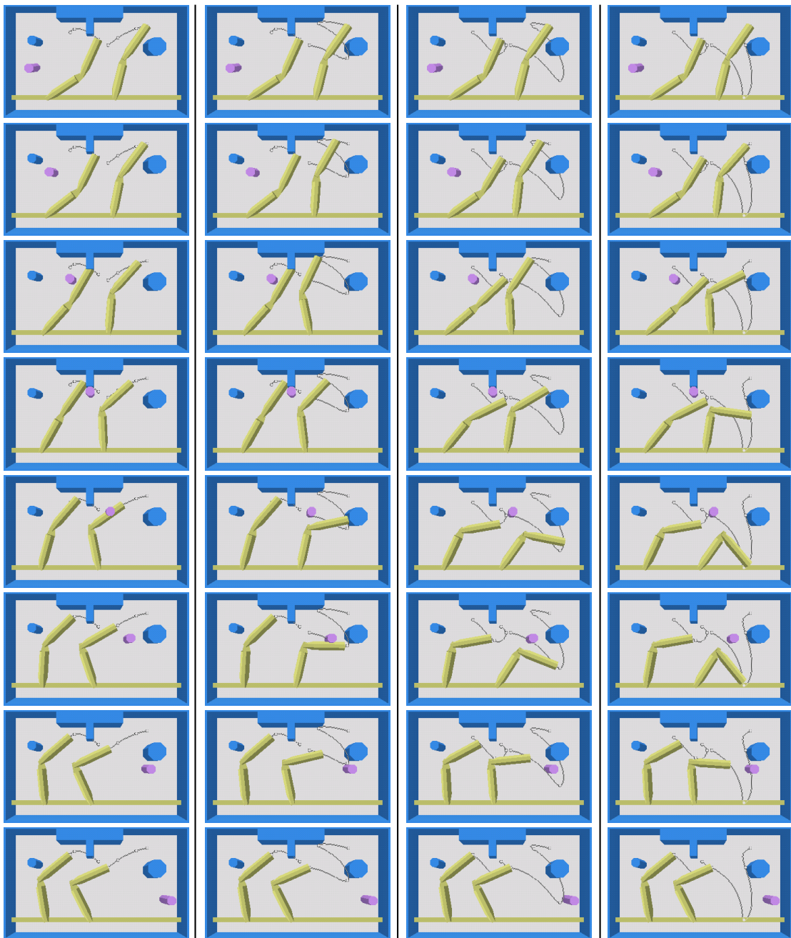
Figure 8.4: A four step planning sequence for the 6 degrees of freedom robot.
