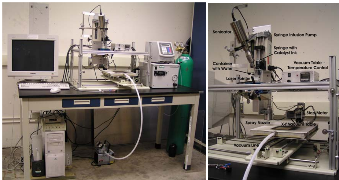
Figure A1: Spray setup for carbon supported platinum catalyst at LANL.
