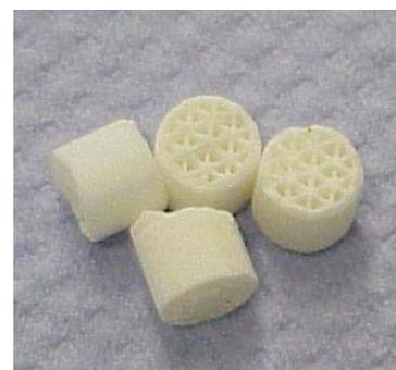
**Fig. 4.1:** Monolith from Sasol with triangular channels.
