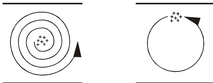
Figure 3. The incoherent ion cyclotron motion is converted, by excitation, into detectable coherent motion. 6
