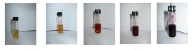
0 min 2 min 5 min 10 min 30 min Figure 4-12. Color change during polymerization.
