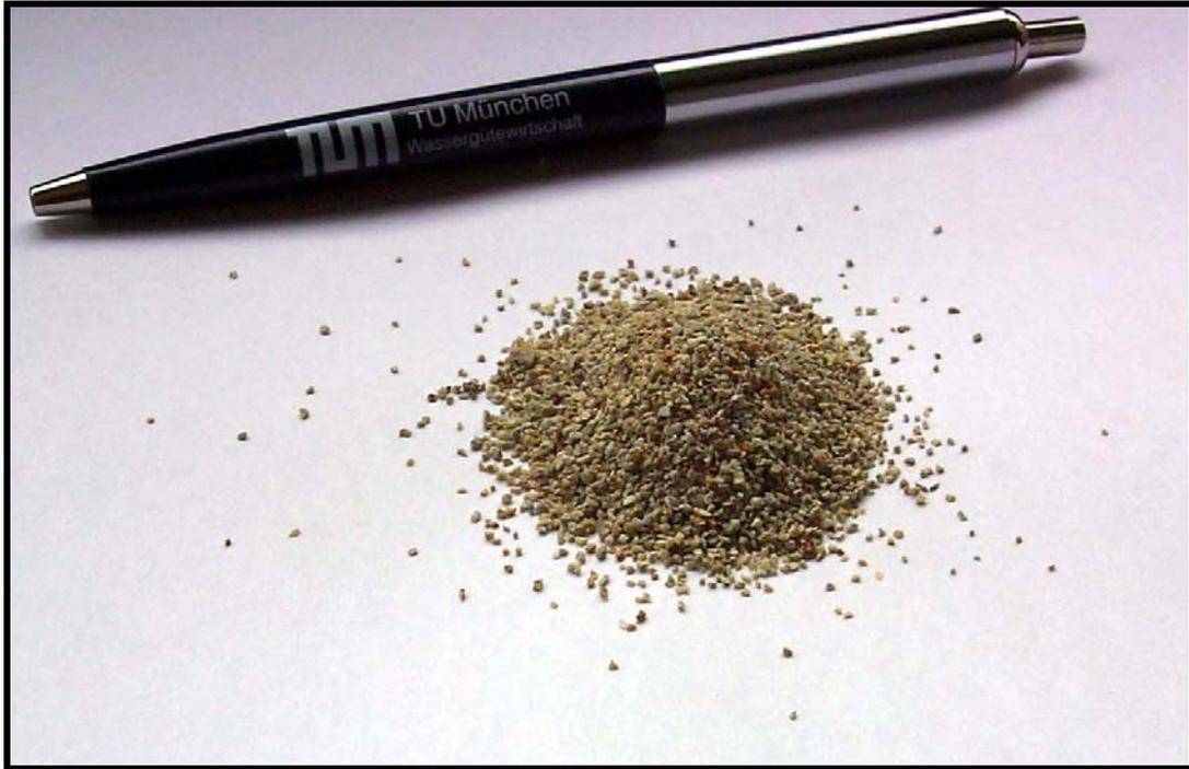
**Figure 14:** Photo from clinoptilolite with a grain size between 0.5 and 1.0 mm.
